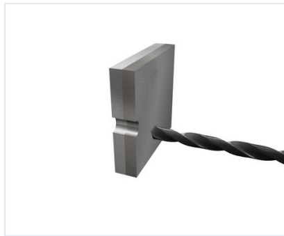
01 Drill starting hole
