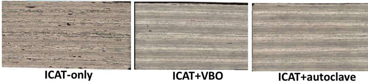
Figure 6: Photomicrographs of IM7/PEKK Panel A (ST = 525°C, TT = 180°C, V = 25 mm/s).
