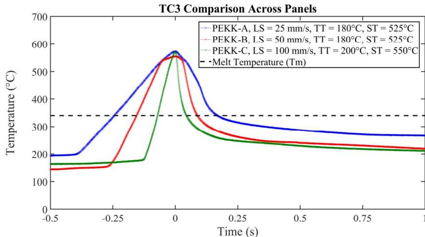
Figure 12: Comparison of times above melt temperature at TC3 located at the center ply for IM7/PEKK Panels A, B, and C.
