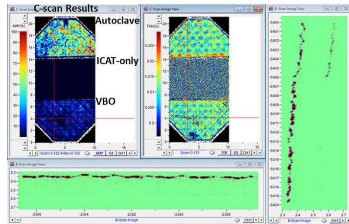
Figure 11: NDI results of IM7/PEKK Panel C (ST = 550°C, TT = 200°C, V = 100 mm/s).
