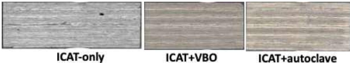
Figure 4: Photomicrographs of T800/PEEK Panel (ST = 500°C, TT = 120°C, V = 100 mm/s).
