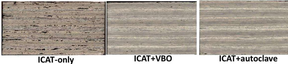
Figure 7: Photomicrographs of IM7/PEKK Panel B (ST = 525°C, TT = 180°C, V = 50 mm/s).
