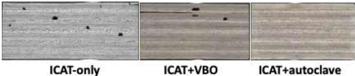
Figure 5: Photomicrographs of IM7/LM-PAEK Panel (ST = 450°C, TT = 80°C, V = 400 mm/s).
