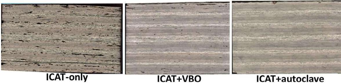
Figure 8: Photomicrographs of IM7/PEKK Panel C (ST = 550°C, TT = 200°C, V = 100 mm/s).
