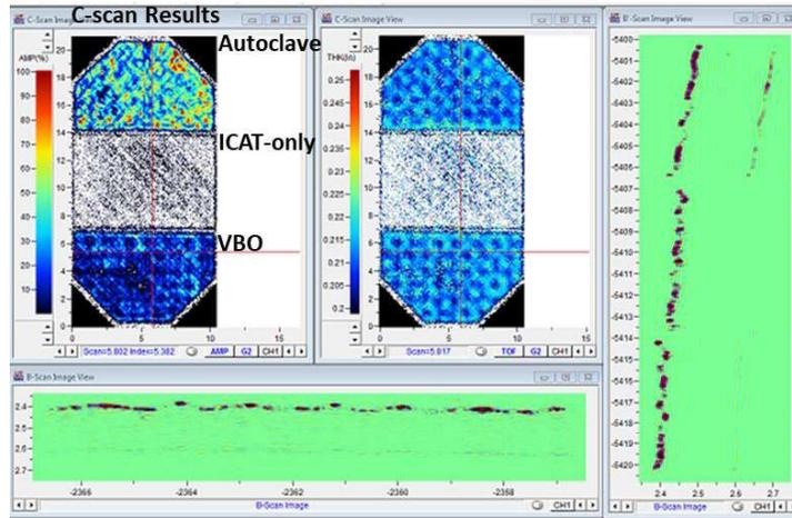
Figure 9: NDI results of IM7/PEKK Panel A (ST = 525°C, TT = 180°C, V = 25 mm/s).
