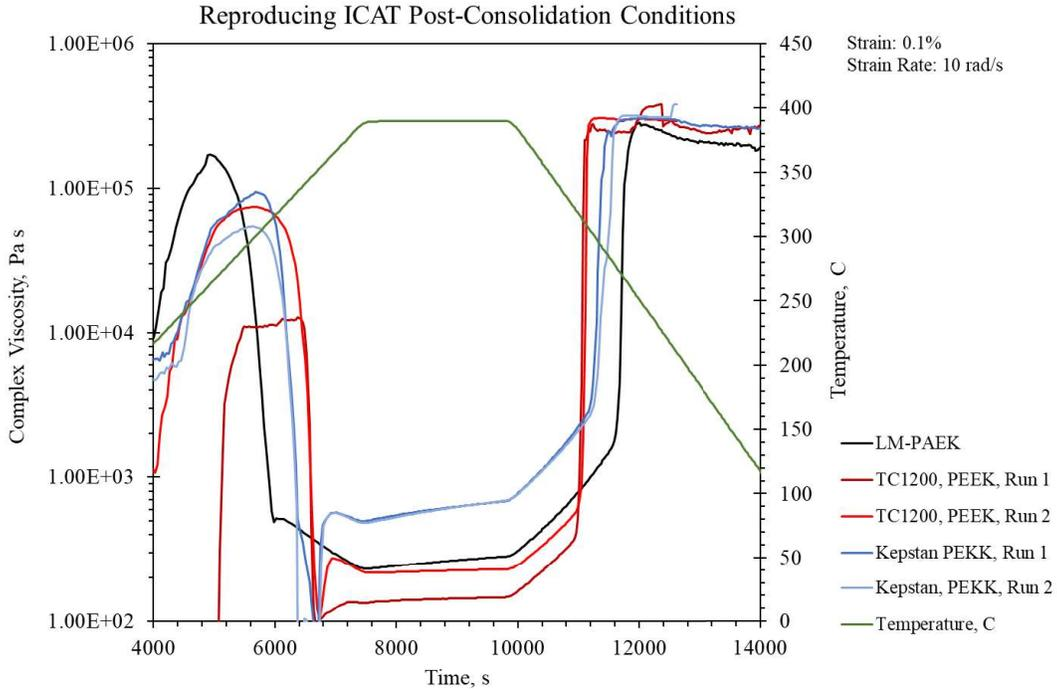
Figure 3. Parallel plate rheology of PEEK, LM-PAEK, and PEKK neat polymers using the supplier recommended PEEK autoclave processing temperature (390°C).
