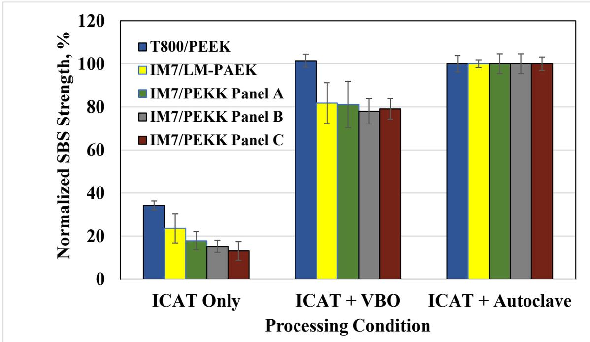
Figure 13: SBS results normalized to the “ICAT + autoclave” values from T800/PEEK, IM7/LM-PAEK, and IM7/PEKK “ICAT-only” and “ICAT + post processing” panels.
