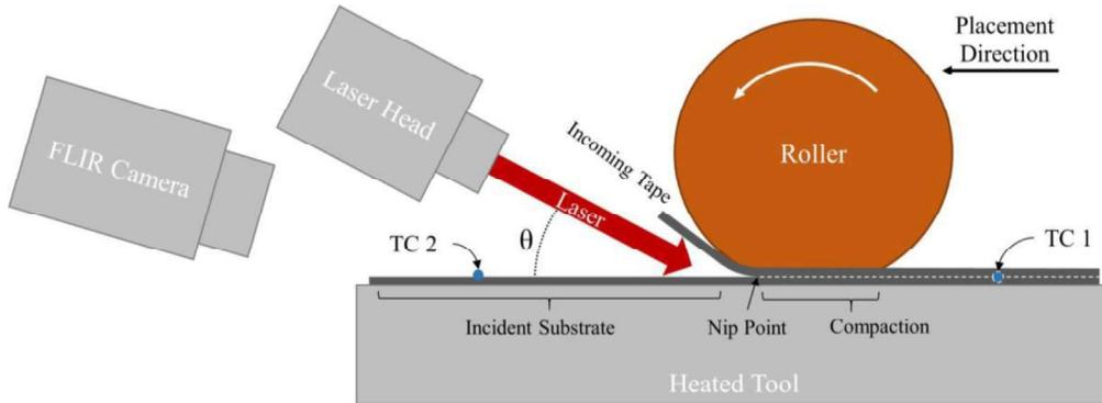
Figure 2: Schematic diagram of laser-assisted AFP.
