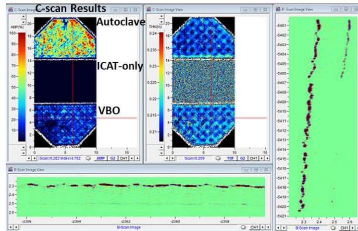
Figure 10: NDI results of IM7/PEKK Panel B (ST = 525°C, TT = 180°C, V = 50 mm/s).
