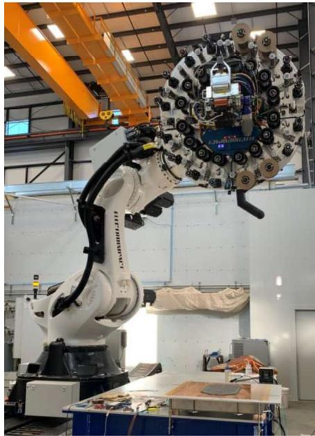
Figure 1: Electroimpact<sup>®</sup> six-axis AFP robot arm (Image Credit: Electroimpact, Inc.<sup>®</sup>).
