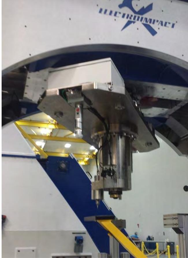
**Figure 14: Electroimpact Modular Ultrasonic Cutting / Probing Head. Ultrasonic knife on the left, touch probe interface on the right. The touch probe itself is not present.**
