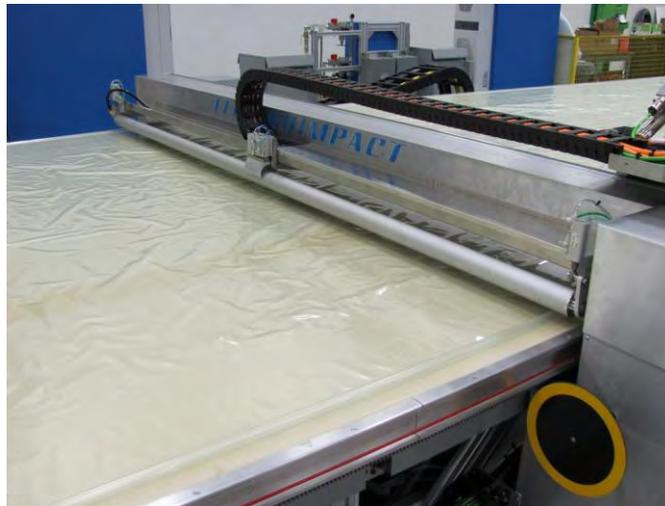
Figure 6: Rear view of Ultrasonic Cutting Gantry showing backing film pickup mechanism.
