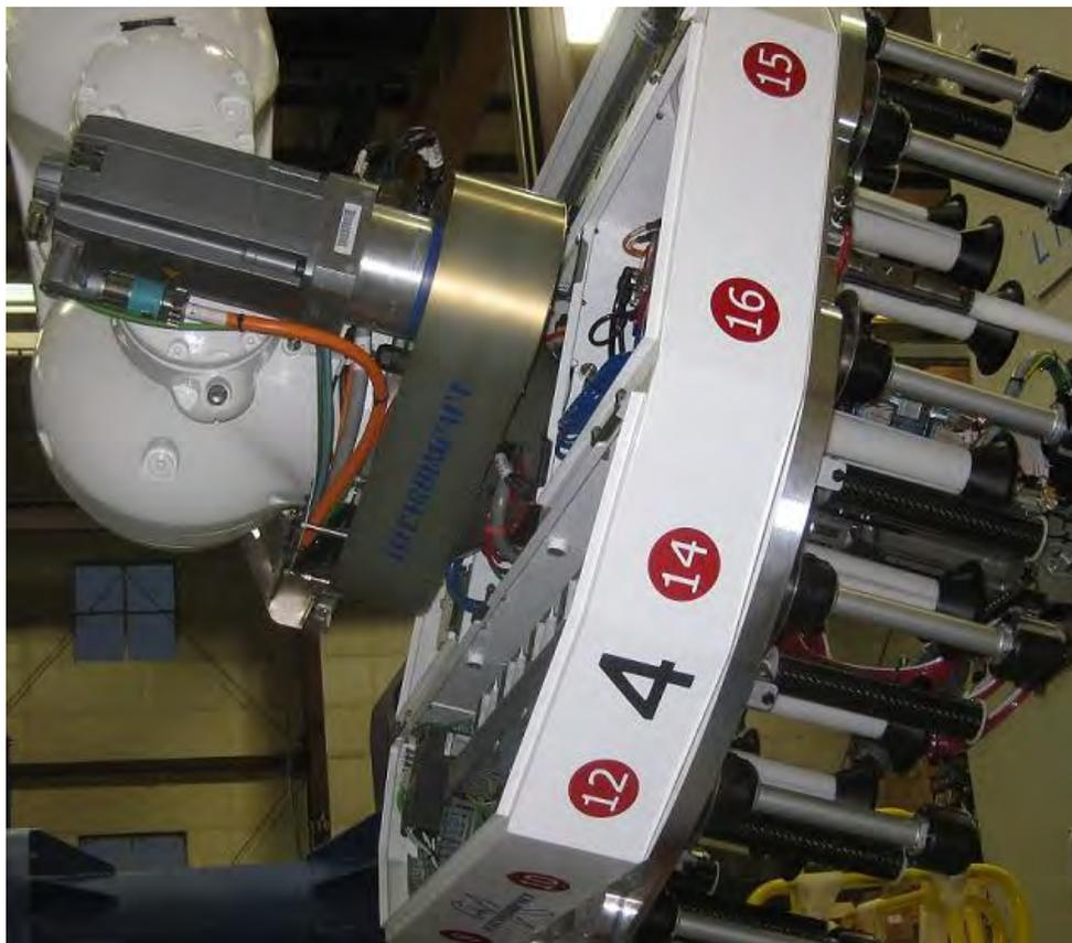
Figure 10: High speed Axis 6 (C-Axis) retrofit.
