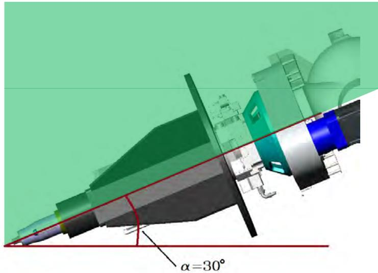
**Figure 15: Rendering of High Clearance Ultrasonic Cutting Head at 30° from horizontal. Operating range shown in green.**
