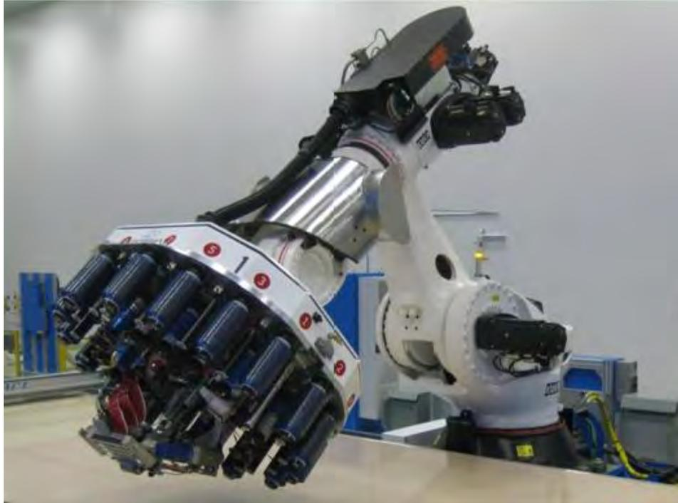
**Figure 9: Modular AFP Head on Accurate Robot.**
