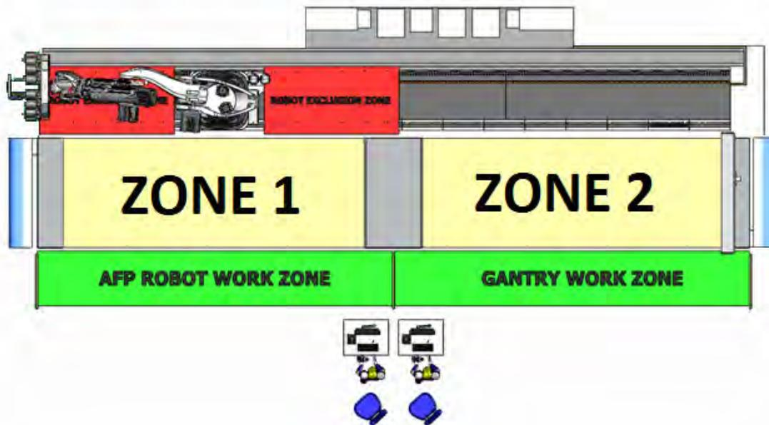
Figure 4: Work cell divided into two zones.
