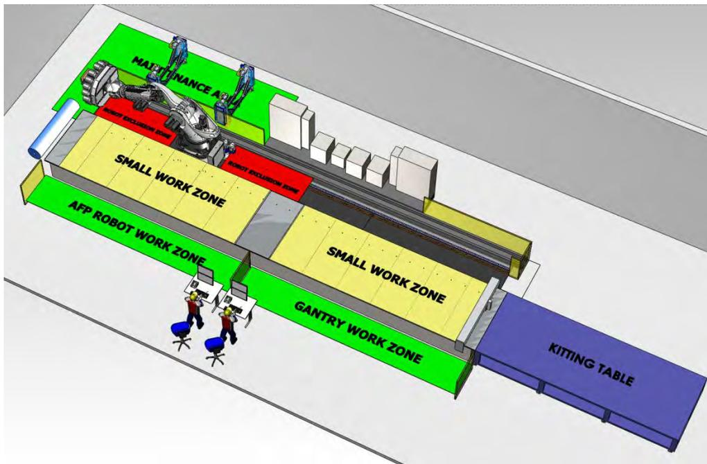
Figure 13: Example of safe zone configuration: Ultrasonic Cutting Gantry and AFP Robot Parked.
