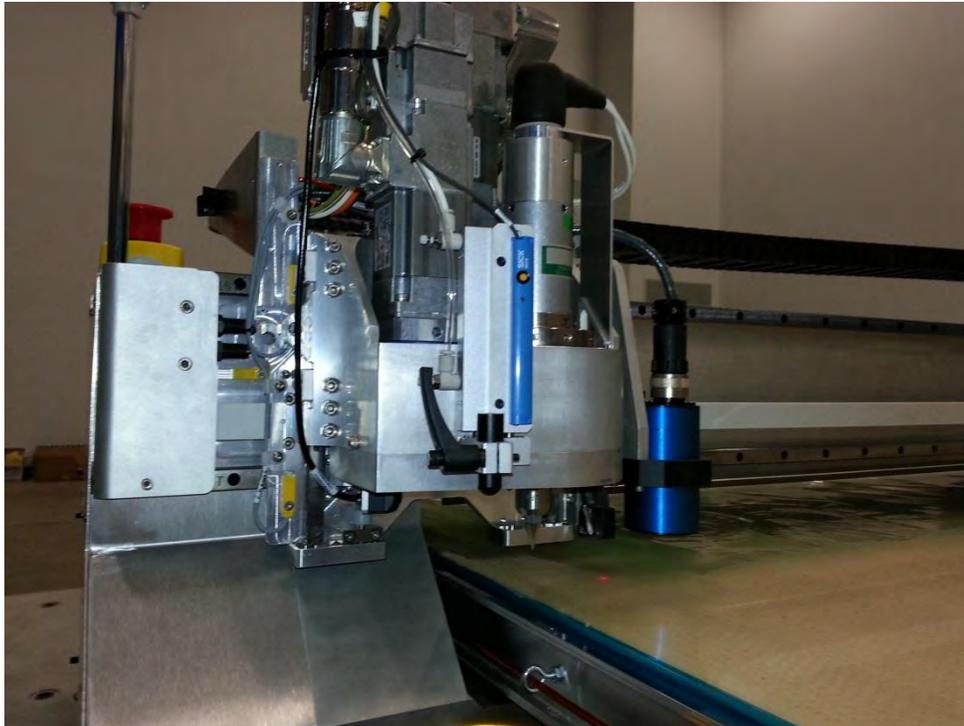
**Figure 7: Close-up of process head. Tools from left to right: Toolpoint Camera, Table Mapper, Ultrasonic Knife, Contrast Sensor, Inkjet Printer.**
