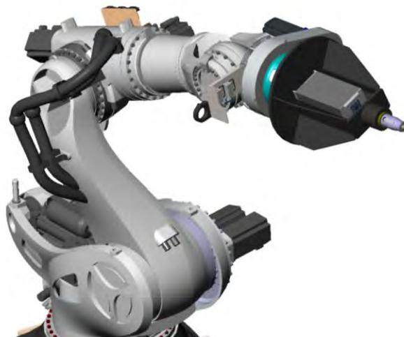
**Figure 16: Rendering of High Clearance Ultrasonic Cutting Head on Accurate AFP Robot**
