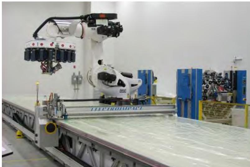
Figure 1: Ultrasonic Cutting Gantry, Vacuum Table, AFP Robot.
