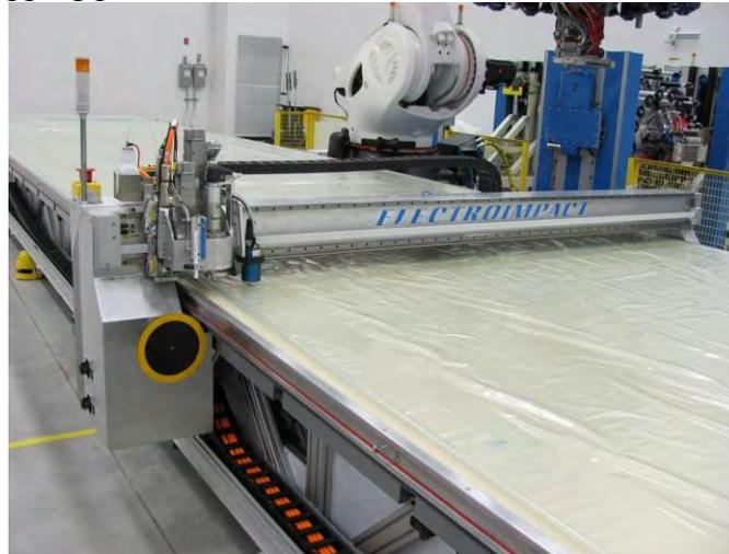
Figure 5: Front view of Ultrasonic Cutting Gantry showing main process head.
