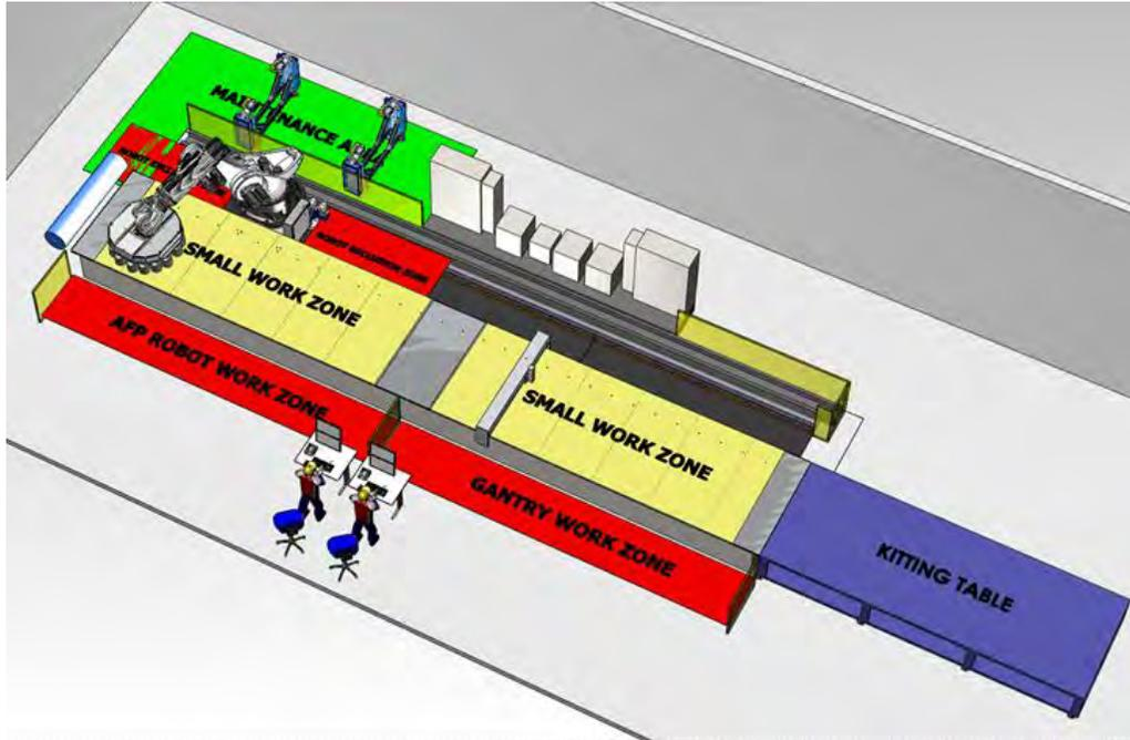
Figure 12: Example of safe zone configuration: Both Ultrasonic Cutting Gantry and AFP Robot working.
