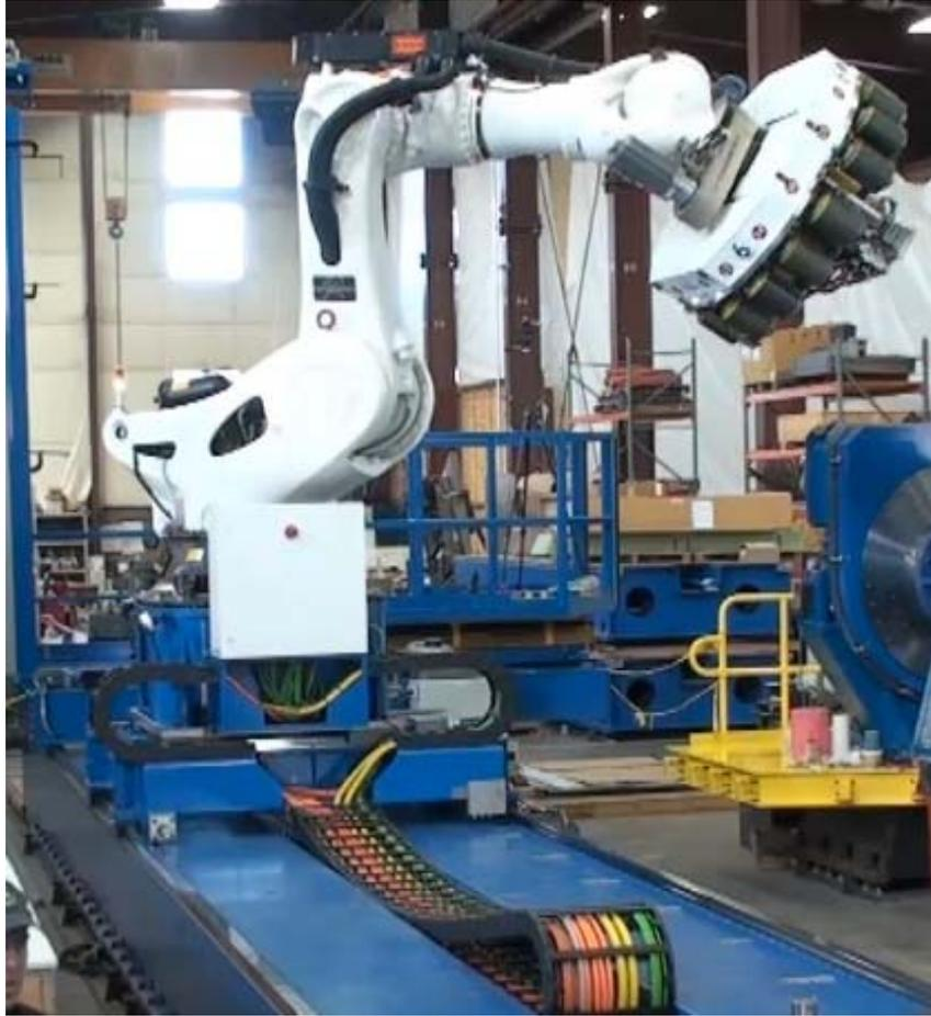
Figure 10. Fiber placement robot with axis 6 retrofit, rotators, and dual linear axes under the robot base.
