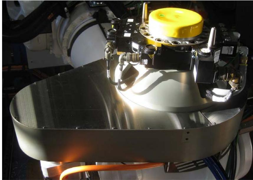
Figure 5. Complete Electroimpact designed axis 6 assembly.
