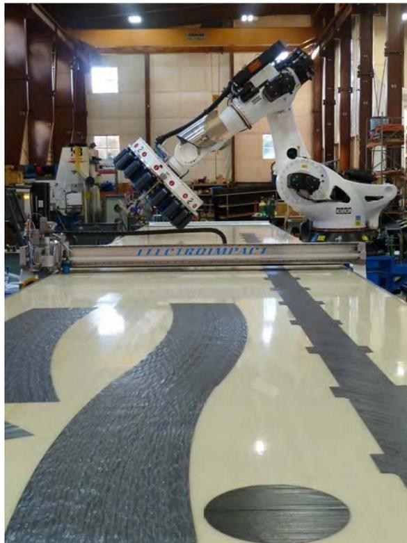
Figure 12. Typical flat charges on the vacuum table.
