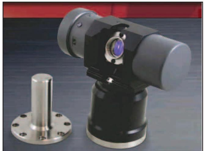
**Figure 3.** The Active Target replaces a conventional SMR and automatically adjusts to keep pointing at the tracker
