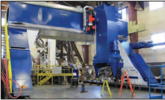
**Figure 6.** Large gantry automated fiber placement machine undergoing volumetric compensation—note tracker directly underneath machine. A 1.5-m-thick foundation poured on compact fill ensures a stable instrument station even under this heavy load.
