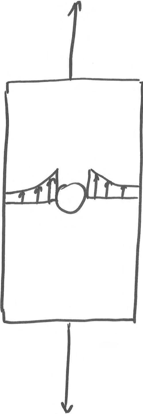
This is bad – a 20% increase in load will cut fatigue life in half. Enter the coldworked hole with this stress distribution -
