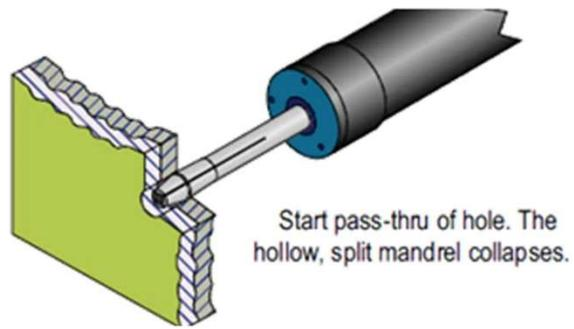
Start pass-thru of hole. The hollow, split mandrel collapses.
