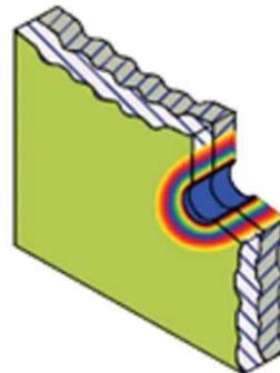
With no sleeve to discard, the hole has been coldworked.
