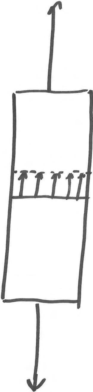
This gives us a nice, even stress distribution – easy to understand and analyze. Unfortunately, a lot of aircraft structures don't look like this, they are full of holes that tie them to the next part in the load path. Pulling on a piece of metal with a hole in it gives us a stress distribution with more stress at the
