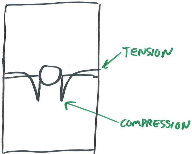
It has a locked in compressive stress at the edge of the hole, perfect for counteracting the higher stress at the edge of the hole from external loading. Combining the 2 states of stress, we get a more even
