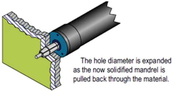
The hole diameter is expanded as the now solidified mandrel is pulled back through the material.
