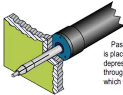
Pass-thru is complete. Nosecap is placed flush to material. After depressing trigger, the pilot extends through center of hollow mandrel, which solidifies.
