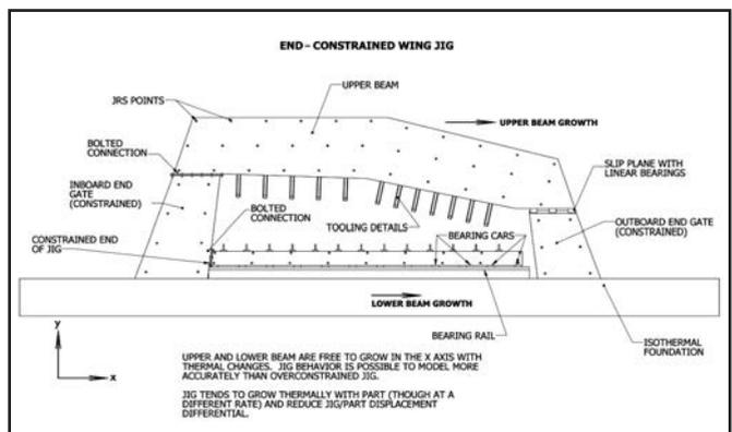
Figure 4. End-constrained wing jig
