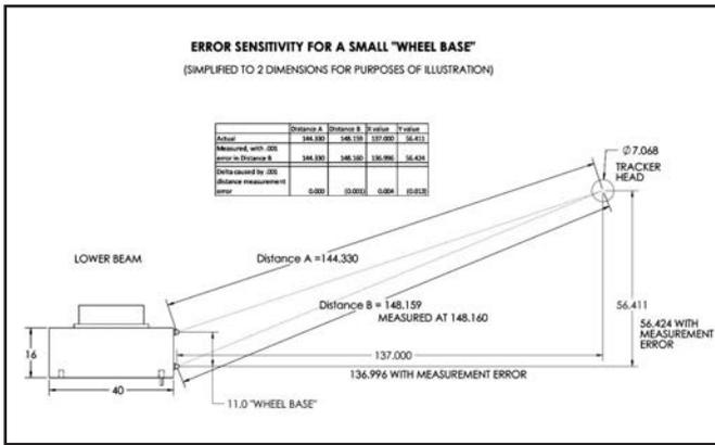
Figure 7. Error sensitivity for a small “wheel base” is very high
