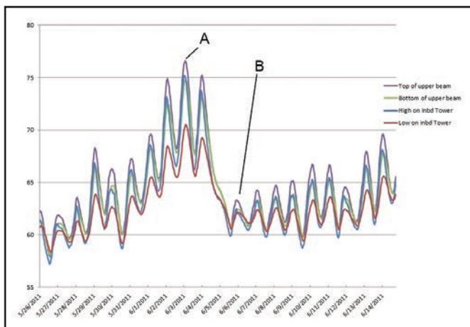
Figure 9. Temperatures varied by nearly 20° F over three weeks, as hourly monitoring shows; note change in temperature spread between points A and B, indicating a varying vertical thermal gradient
