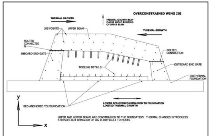
Figure 3. Thermally overconstrained jig
