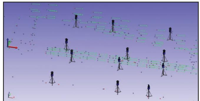
Figure 6. A vector plot shows the difference between including and excluding the outboard end gate from the JRS bundle
