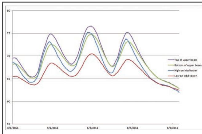
Figure 10. Hourly temperature recordings indicate a daily temperature swing of nearly 8° F.
