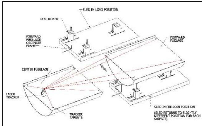
Figure 7. Schematic showing tracker and target positioning
