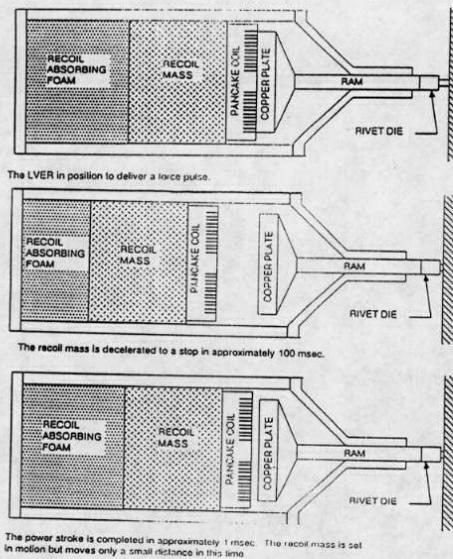
Figure 2: Operating Sequence of the LVER Recoil Control System
