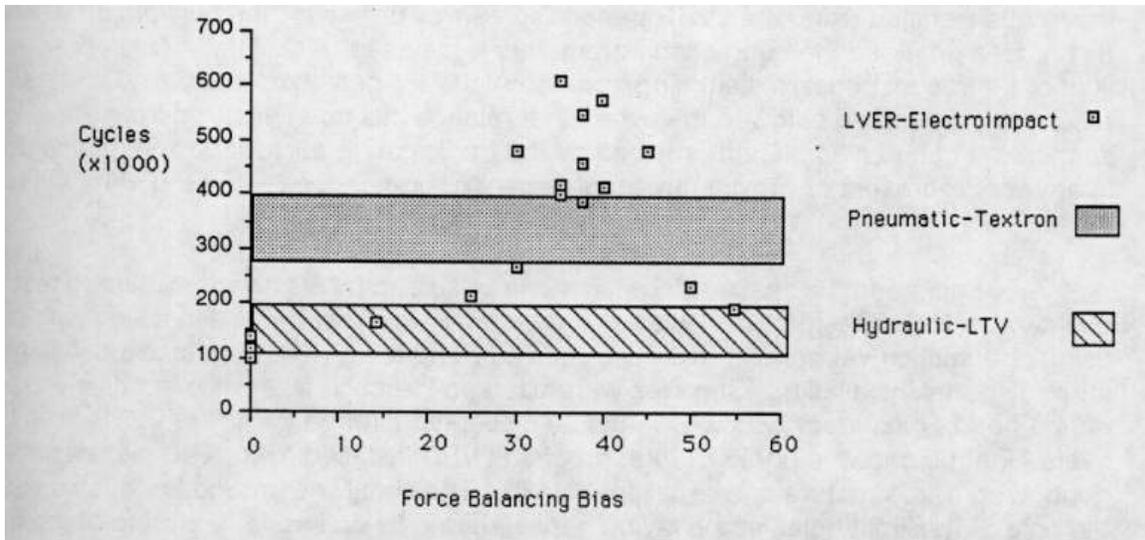
Figure 7: Effect of Force Balancing Bias on fatigue life for 7050 Briles countersunk rivets in .142" stack up. Test run at 24 ksi maximum stress with a .05 load ratio.
