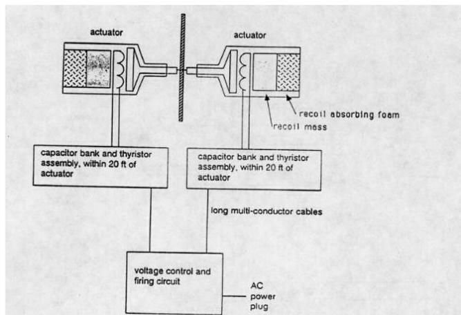
Figure 1: LVER Block Diagram
