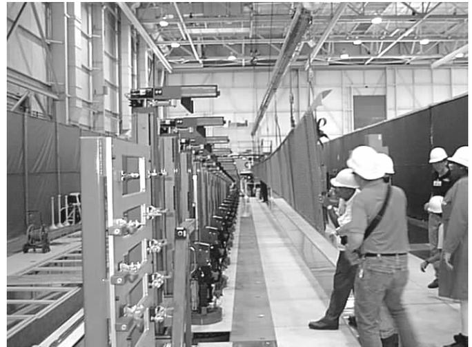
Figure 6: Loading Spar into Fixture
