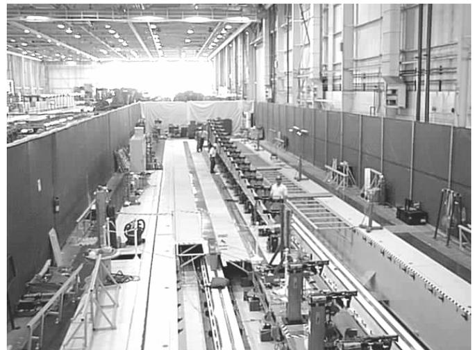
Figure 7: Spar Loaded in Fixture
