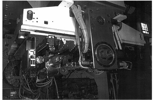
Figure 2: Clamp Table with Process Tools
