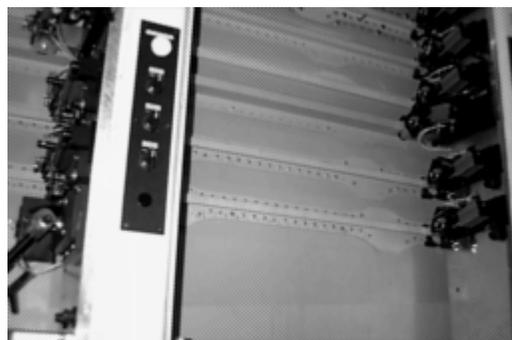
Figure 8: E4000 installs offset fasteners
