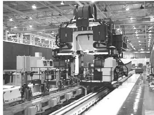
Figure 6: Loading Spar into Fixture
