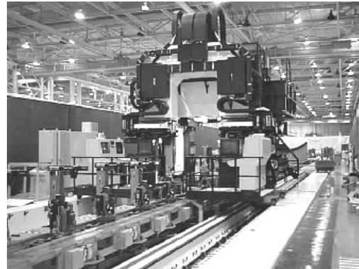
Figure 2: Clamp Table with Process Tools
