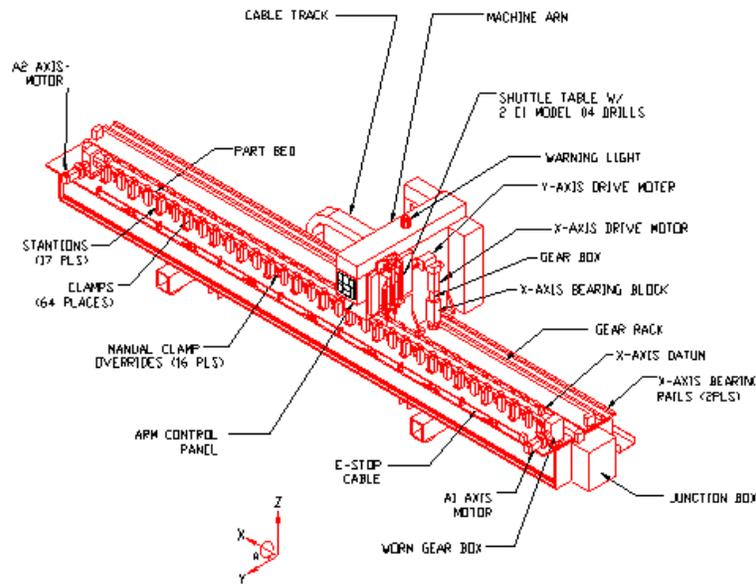
Figure 2. - The Automatic Stringer Drilling System
