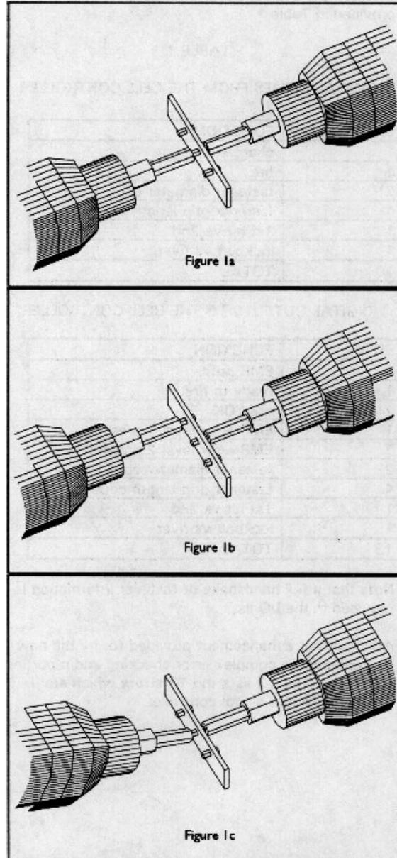
Figure 1 Proper (a) and incorrect alignment (b, c) of handheld EMRs
