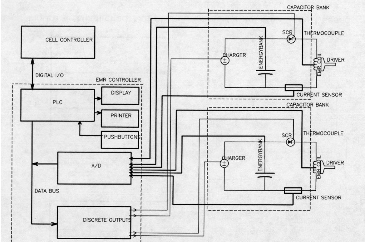
Figure 5 Digital EMR block diagram
