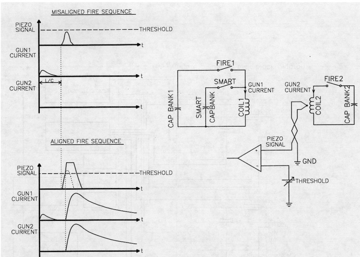
Figure 4 Misaligned and aligned signal output from smart sensor
