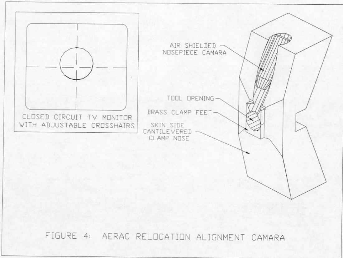
FIGURE 4: AERAC RELOCATION ALIGNMENT CAMARA
