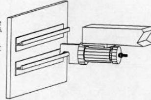
6. AN M52 IS USED TO MOVE THE OFFSET TOOLING INTO POSITION TO ENTER THE STRINGER. THIS M-CODE TURNS ON THE FLYING HEIGHT TRACER, NULLS IT OUT, TURNS IT OFF, AND RETRACTS THE TOOLING  $3/16$  INCH.
