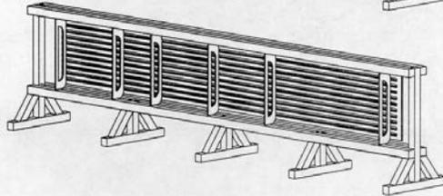
THE OPERATOR OPENS A FINAL BAY AFTER FORMBOARDS IN THE SECOND BAY ARE REPLACED. THE PANEL IS REMOVED FROM THE JIG AS A COMPLETED PART AFTER THE RIVETS IN THE FINAL BAY ARE INSTALLED.
