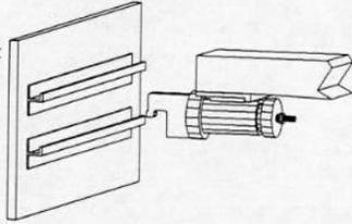
7. THE EDGE DISTANCE TRACER IS TURNED ON WITH AN M55, AND THE OFFSET TOOLING MOVES INTO THE STRINGER. NEXT AN M40 TURNS ON THE FLYING HEIGHT TRACER TO SET THE PROPER FLYING HEIGHT.
