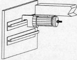
3. THE OFFSET TOOLING IS MOVED OUT OF THE STRINGER USING EITHER AN M45 1' STRINGER CLEAR MOVE, OR A CNC MOVE.
