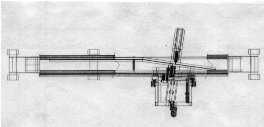
Figure 2 Illustrates the B axis
