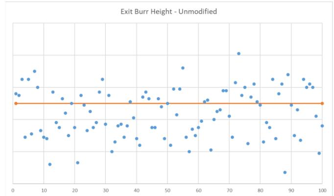
Figure 7: Exit burr height measurements prior to burr shaving.
