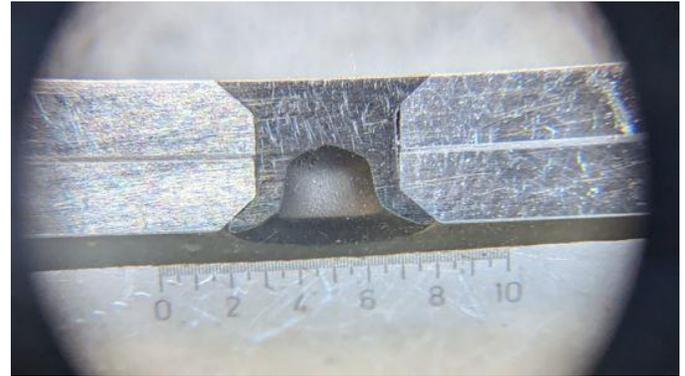
Figure 4: A cross-section of a double flush, hollow tail rivet.
