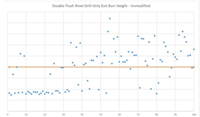
Figure 10: Exit burr height measurements of the drill only holes, prior to intermediate edge breaking.
