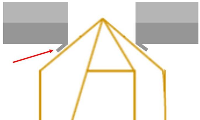
Figure 5: A 100° countersink cutter would sometimes cause exit burrs to fold over, instead of cleanly cutting them.
