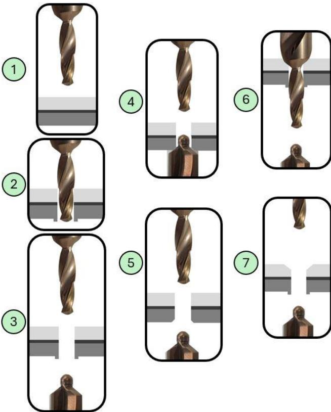
Figure 9: A flow chart of the intermediate edge break process.
