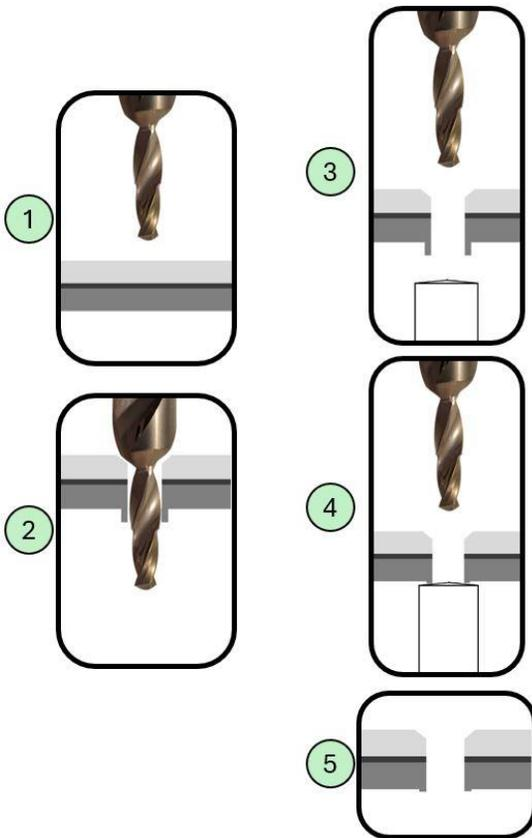
Figure 6: A flow chart of the burr shave process.
