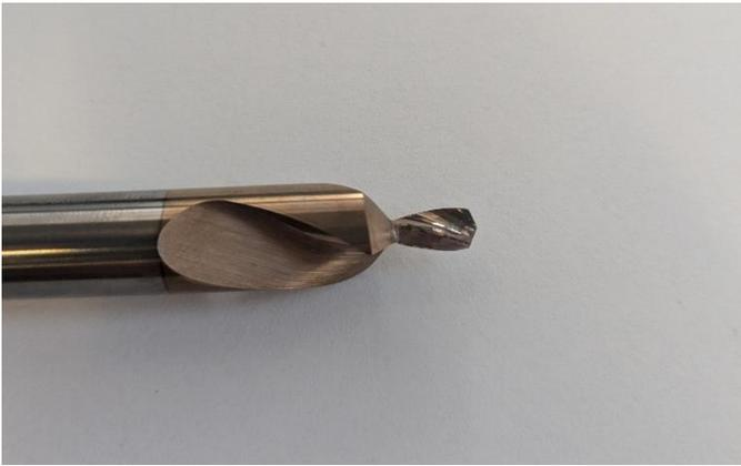
Figure 2: A typical cutter for aerospace manufacturing. The cutter pictured above has a single diameter and countersink geometry for drilling rivet holes.
