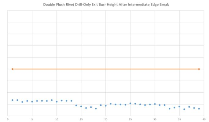
Figure 11: Exit burr height measurements after intermediate edge breaking.
