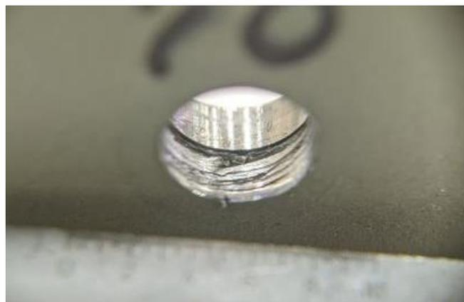
Figure 1: Deep grooves in the aluminum layer from a standard, non-piloted cutter. CRES is on the bottom layer, fiberglass in the middle, and aluminum is on the top layer (closest to the bottom of the image above).
