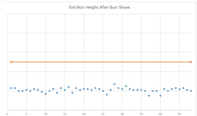
Figure 8: Exit burr height measurements after burr shaving.
