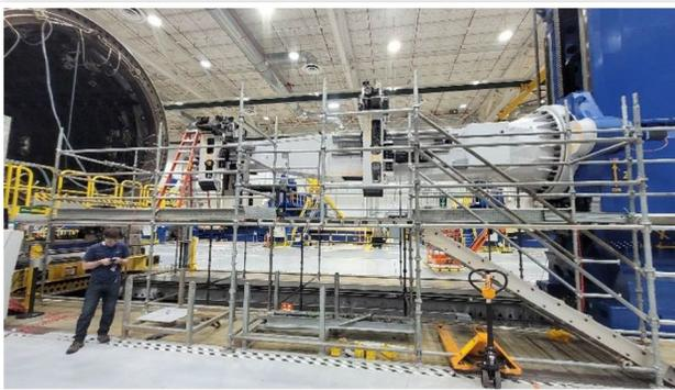
to as a “profile.” These profiles include the following steps: moving each gripper to its nominal location, driving down to the segment, using vision cameras to detect and adjust the grippers, moving to engage the grippers, locking the grippers, using the load cells to induce sideways preload
