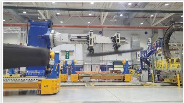
into the grippers, picking up the segment, rotating and performing many small movements to navigate the segment into place, engaging clamps, and finally releasing the grippers. Some segments have only a few steps due to minimal clearance issues, while others require many small, complex movements to avoid obstructions. These steps are dictated by the geometry and sequencing of the segments.
