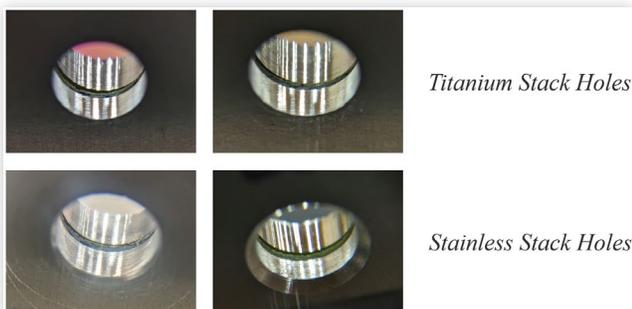
**FIGURE 7** Exit burrs are automatically removed by the fastening machine using an IML-side cutter. The machine is programmed such that the cutter barely makes contact with the material in this process.
