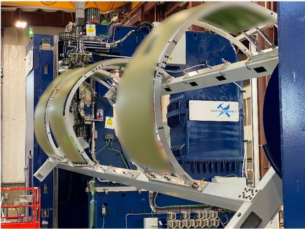
**FIGURE 3** Machine Design Phase Access Study - Panel positioner was overlaid in CAD in many different positions to form a “design constraint cloud” which informed the shape of the lower portion of the fastening machine.
