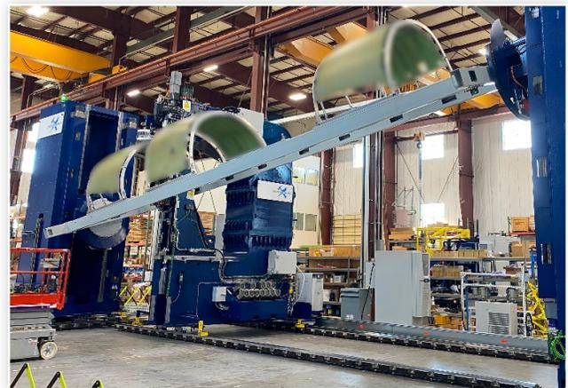
of fastening different types of aircraft parts. Customer requirements also necessitated that the positioning system exhibited the capability of holding an entire shipset (4x fan cowl doors) at once.
