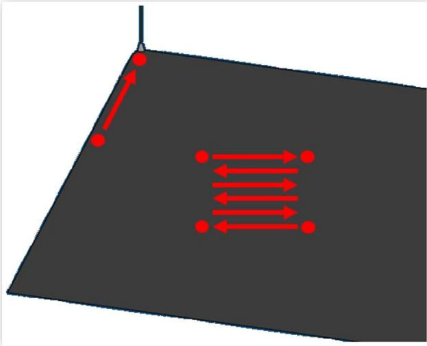
**FIGURE 3** Teach point near collision obstacle.
