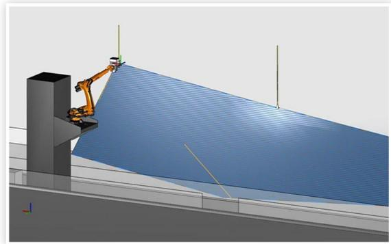
Generated paths are stored as a collection of operations assigned to a given inspection task or part. The technician can put every task in one program to be run all at once or post many programs containing select operations and whatever specific inspection settings are required each operation.
