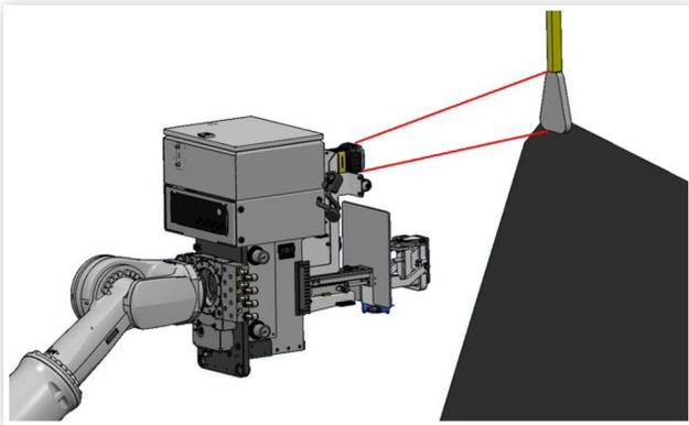
**FIGURE 6** Vision system target acquisition.
