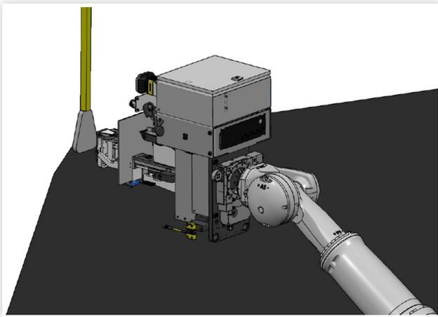
On parts with simple edge contours line generation point-by-point is not overly time consuming. However, a wing panel is huge with curvature in multiple axes. Line scans near edges and collision obstacles are more like splines, requiring many teach points. Additionally the top of the part is seven meters off the factory floor, which means technicians must use a lift to teach scan paths to ensure full-coverage inspection while avoiding collision obstacles.
