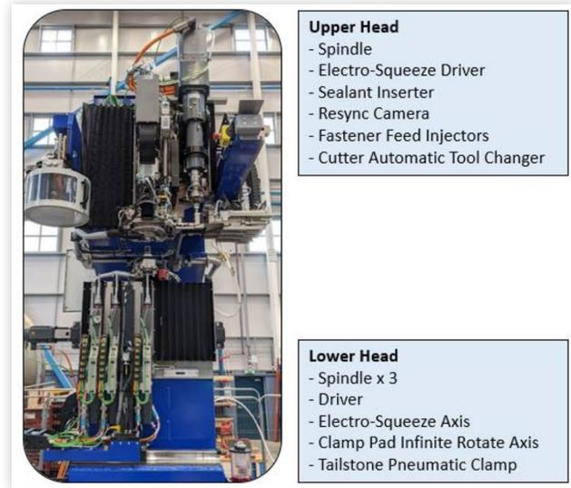
**FIGURE 1** Riveting cell overview
