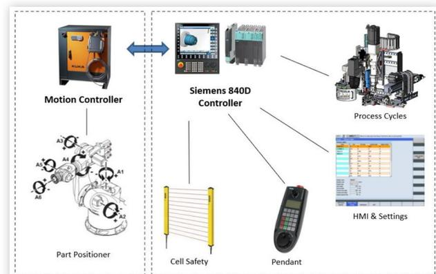
**FIGURE 8** System with single central CNC
