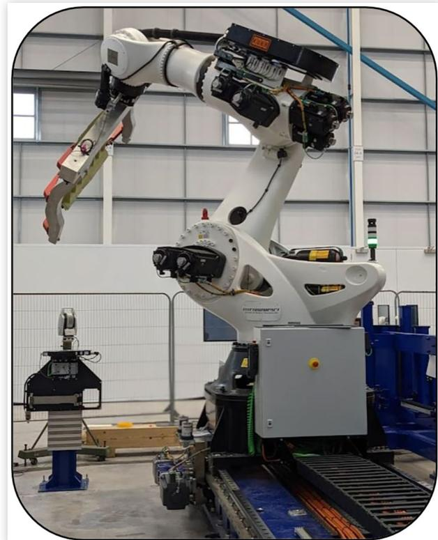
**FIGURE 2** Lower tool servo axis' and process tools
