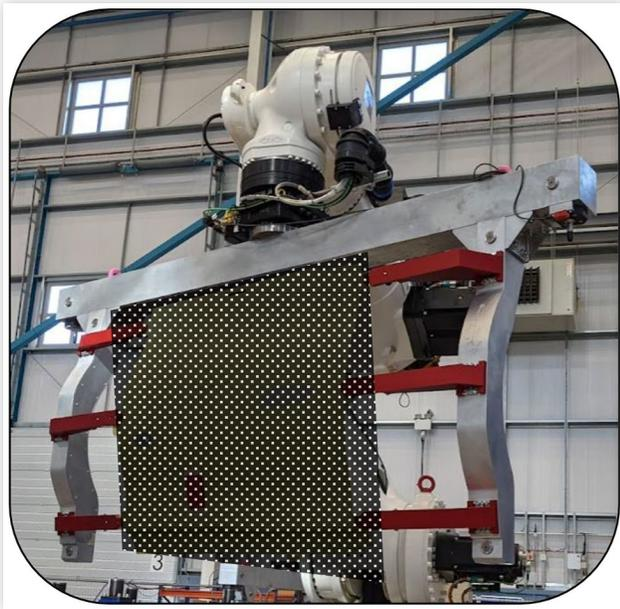
**FIGURE 6** Panel Positioned in C-Frame During Machine Commissioning
