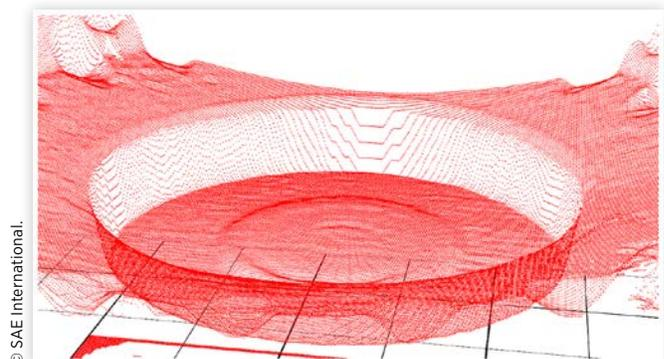
**FIGURE 7** Example of the “knee” inflection points located at the inner diameter of the nosepiece.
