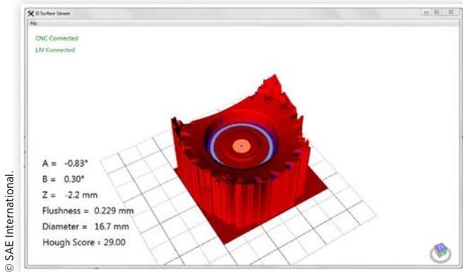
The diameter of the nosepiece is used to cross check that the correct tooling has been installed. The A, B, and Z are used to determine and correct the machine orientation in relation to the panel. The flushness is relayed to the operator and checked to ensure it is within tolerance. And finally the Hough Score is not entirely necessary for the operator, but it gives an example of the circle strength and possible need to clean the nosepiece or the laser.
