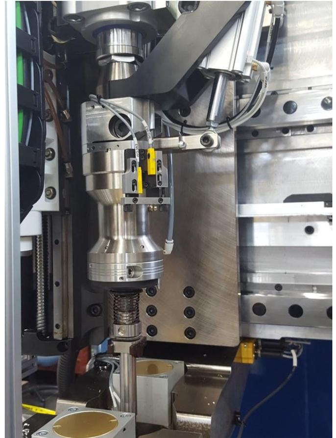
Figure 5: Rivet ram, automatic drawbar and zero clamp
