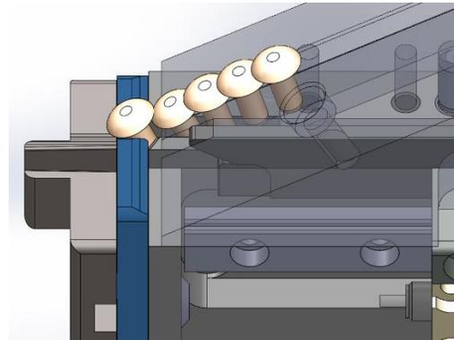
Figure 12: Example of rivets jamming in conventional mini-hoppers
