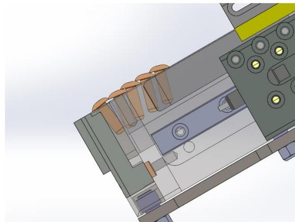
Figure 13: Flexible riveter feeding unjammed rivets
