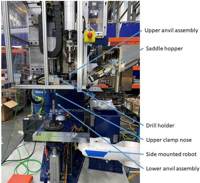
Figure 3: Overview of riveter components
