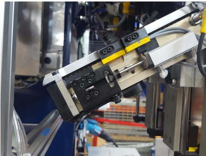
Figure 10: Air cylinder separating rivet
