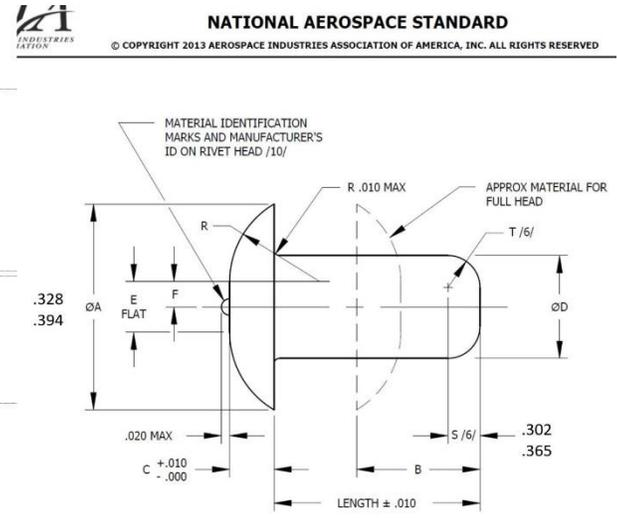
Figure 1: Example of square rivets
