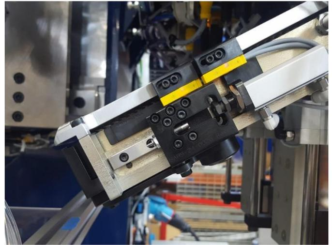
Figure 11: Air cylinder injecting rivet
