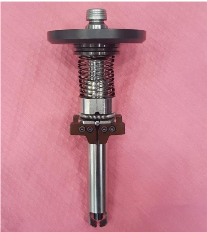
Figure 7: Interior detail of rivet ram showing finger mechanism
