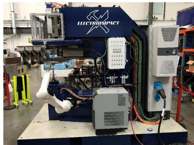
Figure 2: Flexible all electric riveter
