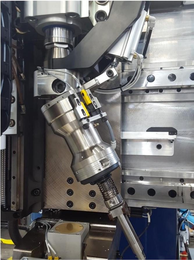
Figure 6: Rivet ram and automatic drawbar
