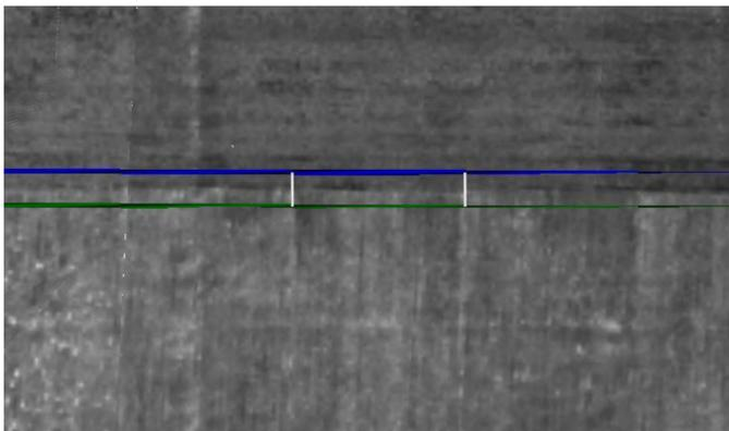
Figure 13. Semi-Automated Ply Boundary Inspection Pass/Fail
