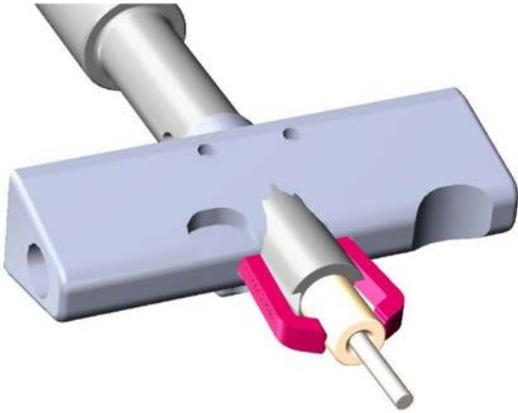
Figure 10. EMR fingers stripped back over the die
