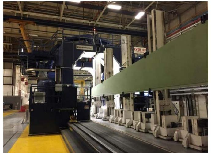
Figure 13. LVER machine with wing panel
