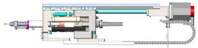
Figure 5. Electromagnetic riveter extended
