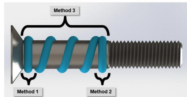
Figure 5. Sealant Methods
