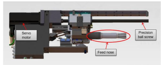
Figure 4. Servo-driven bolt inserter
