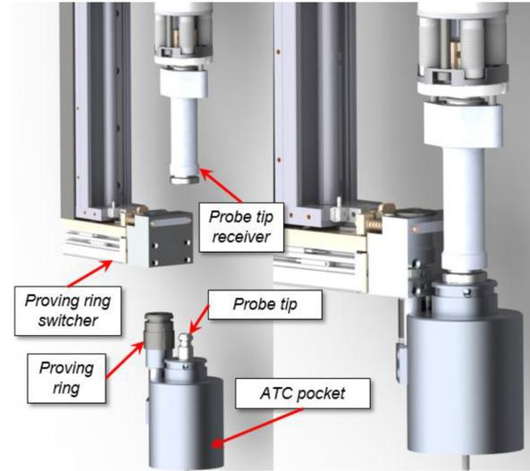
Figure 3. Auto probe and proving ring change
