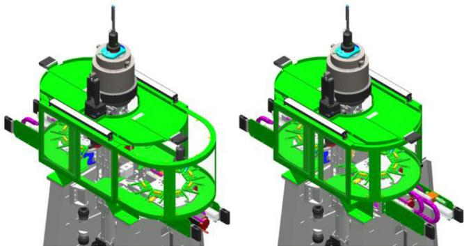
Figure 8. ATC enclosure (depicted here in green), fully encapsulates anvils.
