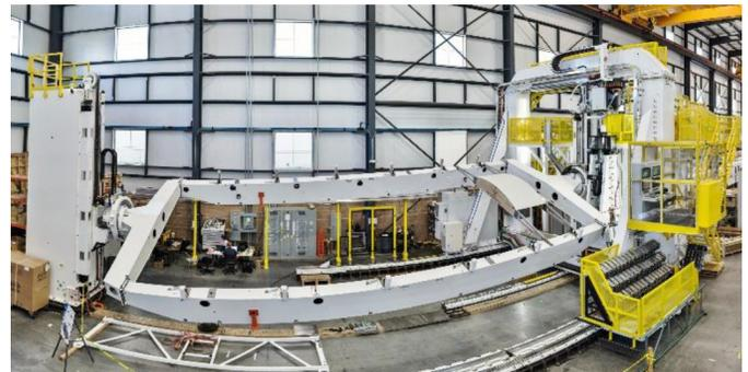
Figure 1. Electroimpact Skin Splice Riveter.
