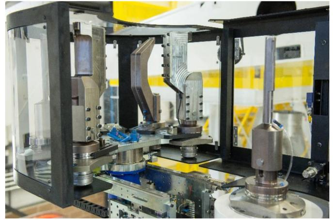
Figure 5. Crescent shaped carousel and fastening head (carousel shown in expanded position)
