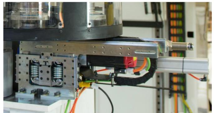
Figure 7. Preloaded springs allowing for vertical compliance
