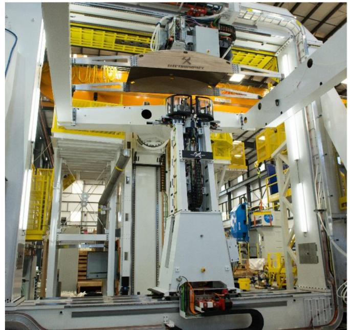
Figure 2. Mounting the ATC directly to the lower fastening head allows the machine to maintain position during tool change.
