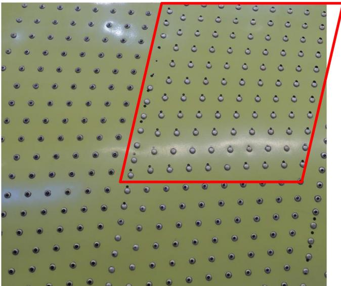
Figure 10. This example of an array of fasteners show areas that needed adjustment (in red) and fastener locations that were correct found during pen plotting.
