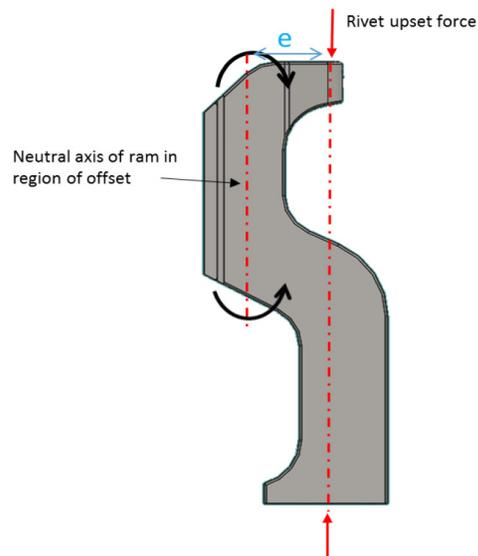
Figure 4. Illustration of internal bending moment applied to offset riveting anvil ram.
