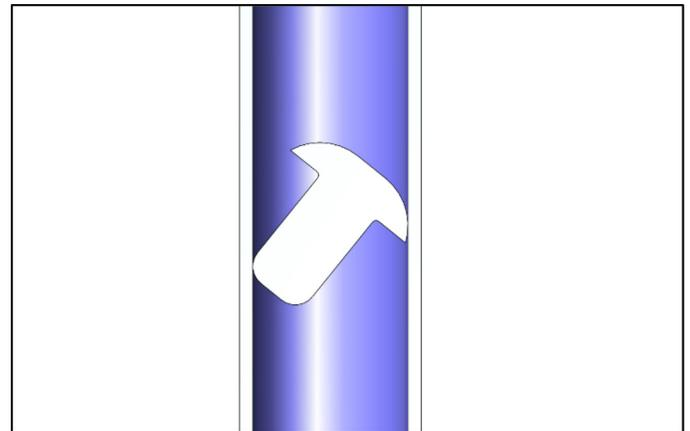
Figure 6. MS20470AD5-4.5 rivet turning in nominally-sized feed tube.
