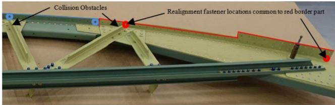
Figure 9. Example of multi-piece bulkhead on C-130. Realignment or resync fasteners are selected for each part.
