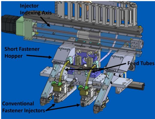
Figure 7. Injector array showing combined hoppers and fastener injectors.
