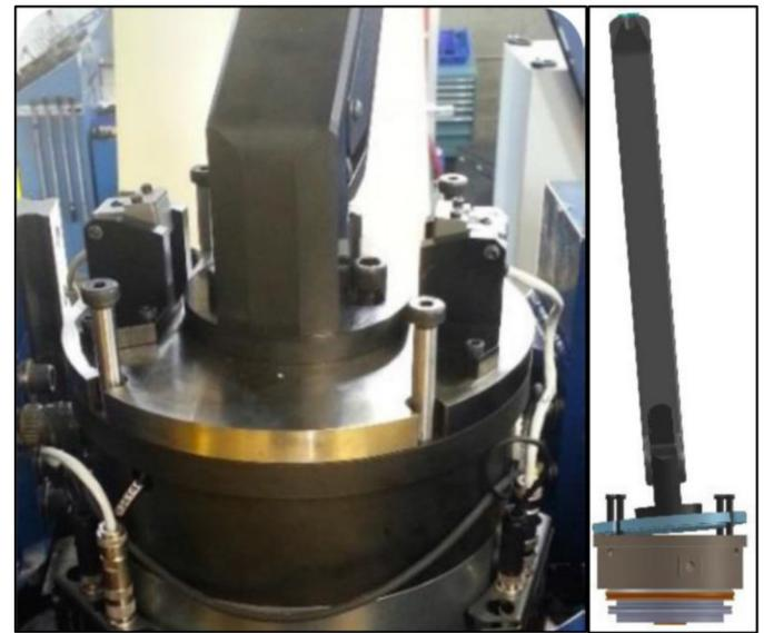
Figure 8. Magnetic lower riveting anvil connection allows separation in the event of a crash.
