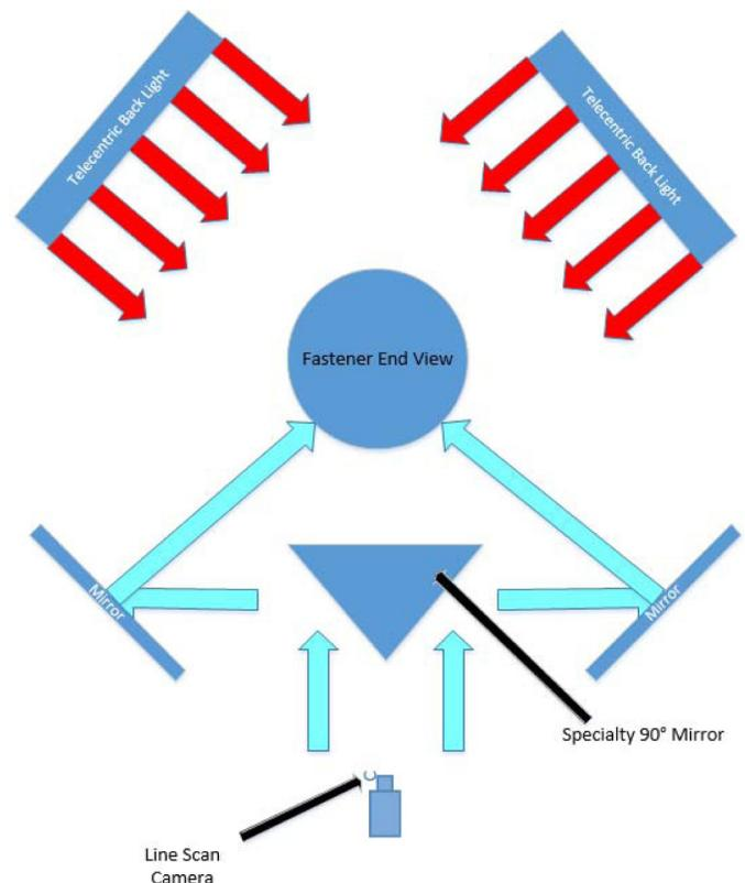
Figure 2. Optical Inspection Layout
