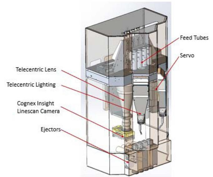
Figure 5. Inspection Assembly
