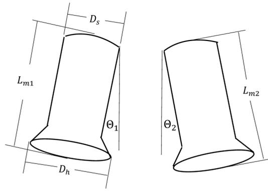
Figure 4. Fastener Measurements In Single Image
