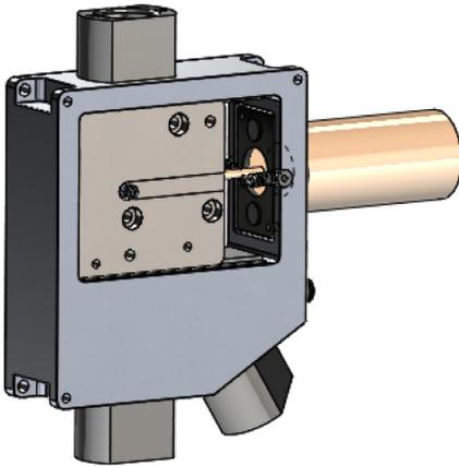
Figure 7. Fastener Eject Actuator Assembly
