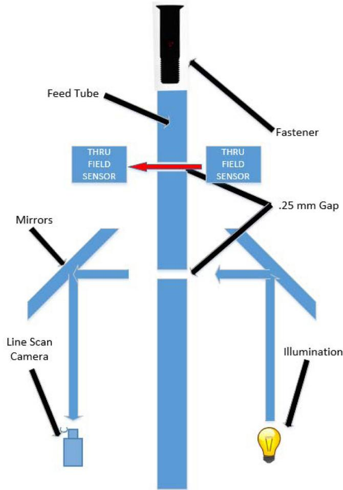
Figure 3. Inspection Method Geometry
