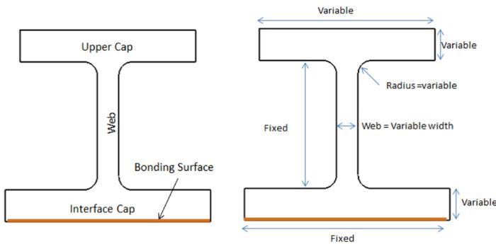
Figure 1. Stringer Cross Section
