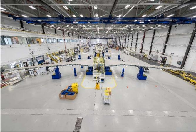
Figure 3 Positions support and locate wing in the LGT020 workcenter. Photo credit: Robert Backus.
