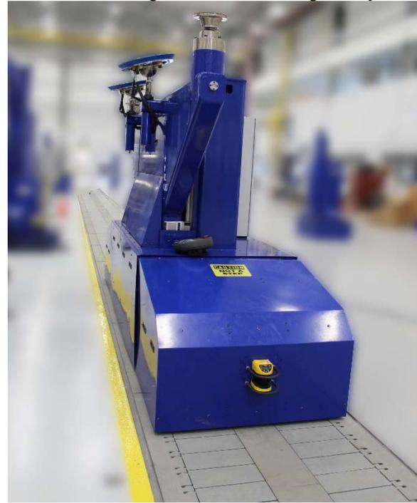
Figure 7: ATLAS with flush to floor interface.
