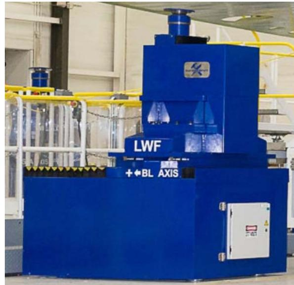
Figure 10: Single positioner module of the APS.
