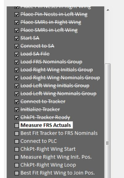
Figure 15: The task list is displayed on the HMI
