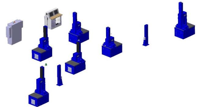
Figure 8: APS layout for wing-to-wing join work center.
