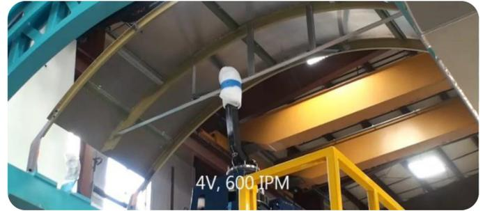
Figure 13. Lower ram hitting part structure during testing
