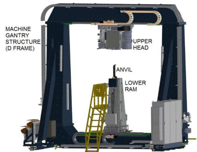
Figure 1. Example of an E7000 D frame riveting machine gantry
