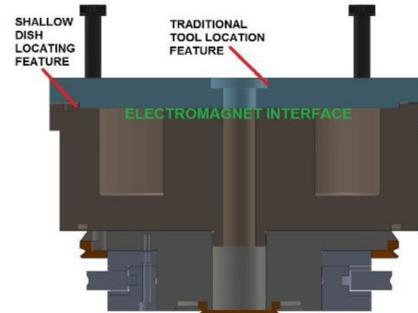
Figure 8. Shallow locating bore detail
