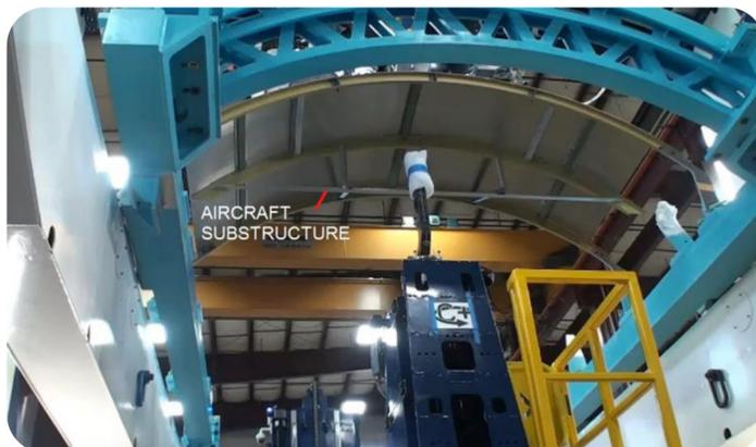
Figure 5. Extended lower ram hitting substructure
