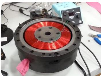
Figure 2. Electromagnet base
