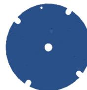
Figure 10. Shoulder screw slots on baseplate
