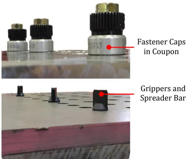
**Figure 11: Fasteners Clamped on Coupon**
