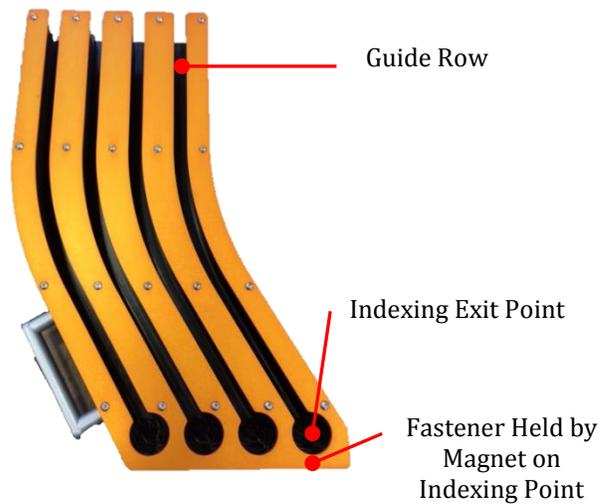
Figure 4: Cartridge Assembly
