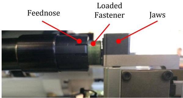
**Figure 9: Loaded Fastener**
