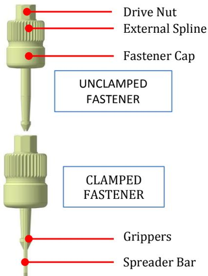
Figure 3: Key Fastener Features
