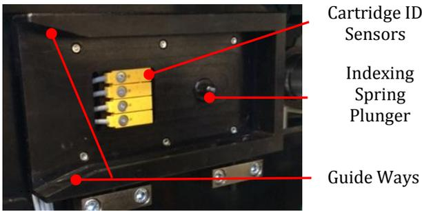
**Figure 5: Cartridge Receiver Assembly**
