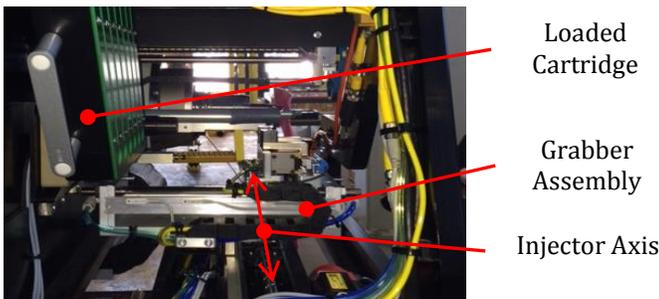
**Figure 7: Injector Assembly Components**
