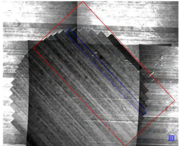
Figure 10. Ply Image with Highlighted Course and Tow.
