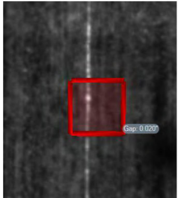
Figure 13. A Single Gap Error.
