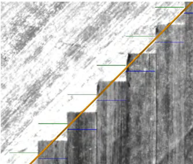
Figure 14. Boundary and tow tolerance highlighting.
