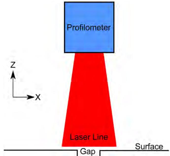
Figure 2. Profilometer Diagram
