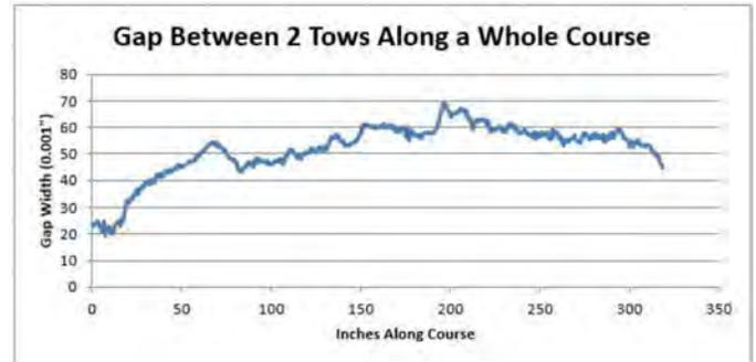
Figure 7. Gap width measured every 0.5" along course direction.
