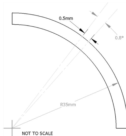
Figure 4. On a highly curved surface, a positional change of 0.5mm can change the angle of the normal vector by 0.8 degrees.
