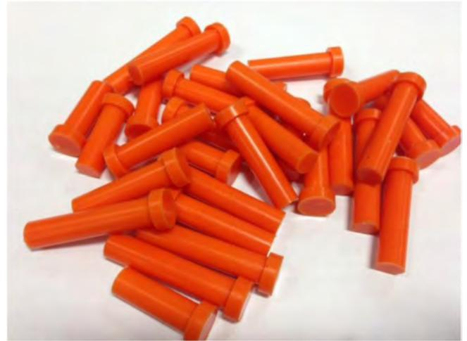
Figure 9. Unheaded injector urethane stop pins
