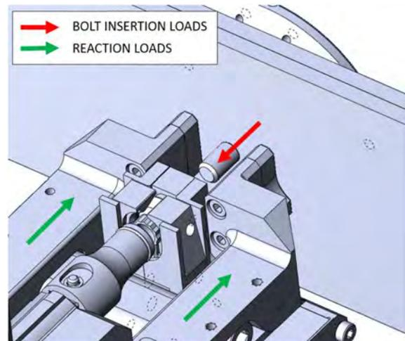
Figure 10. Bolt insertion reaction loads
