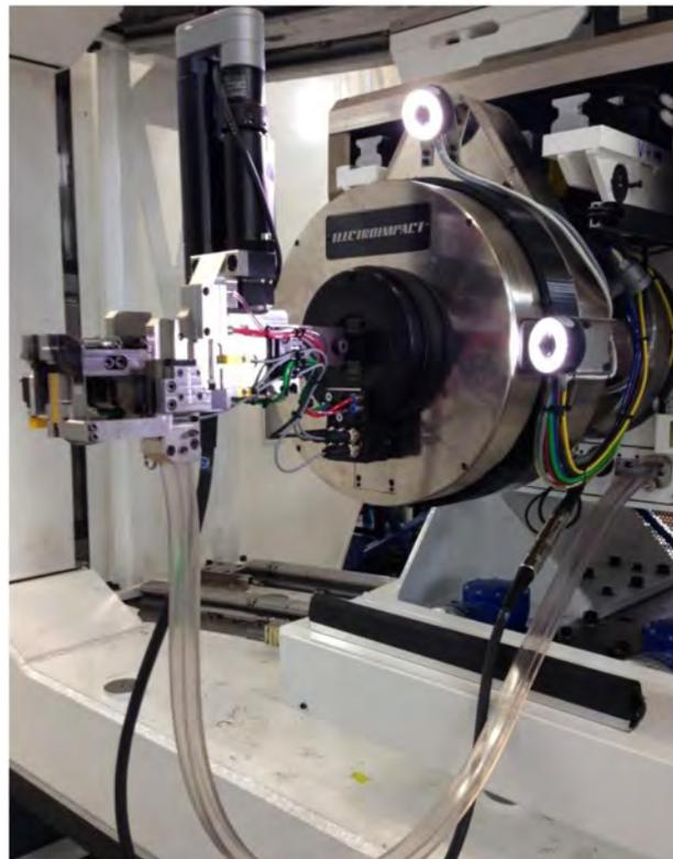
Figure 6. Nut runner anvil installed on PAL machine at Electroimpact
