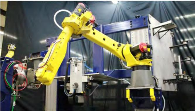
Figure 9. M20 robot at machine socket during a nosepiece tool pickup.
