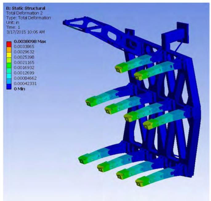
Figure 15. FEA of M20 tool rack indicates 0.003” deflection at tool cradle (yellow to blue differential).
