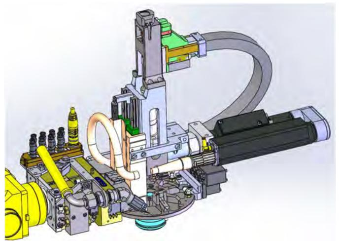
Figure 4. 3/8" nutrunner nosepiece in M20 EOAT
