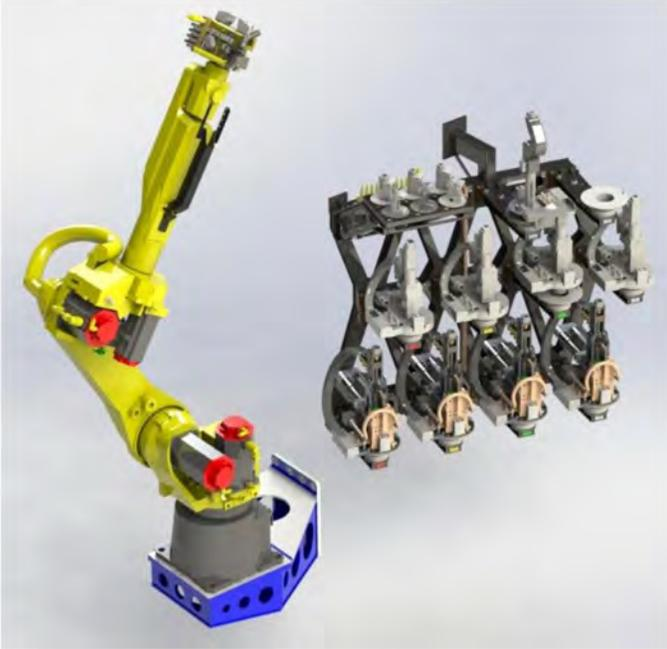
Figure 8. M20 robot with nosepiece rack.
