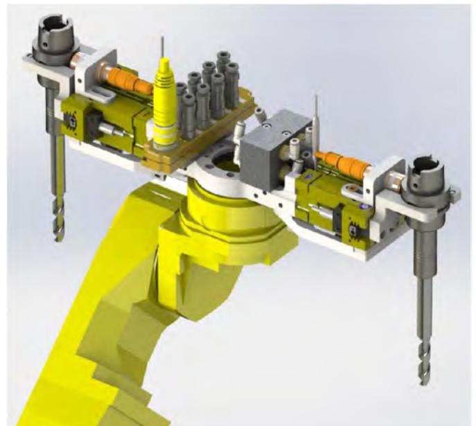
Figure 7. M10 robot EOAT
