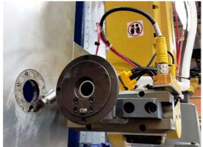
Figure 12. The M20 EOAT cleans a machine tool socket immediately prior to installing the vacuum nosepiece.
