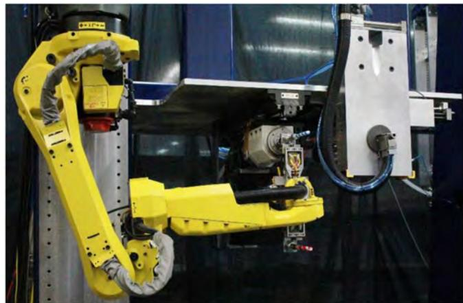
Figure 6. M10 robot at drill spindle during drill bit pickup.
