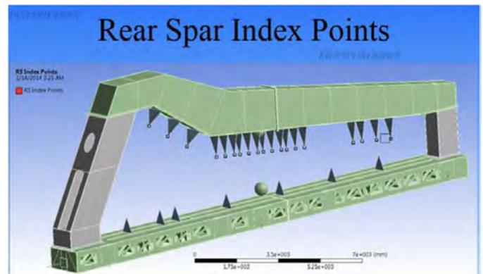
Figure 6. Example tooling index points where results were extracted
