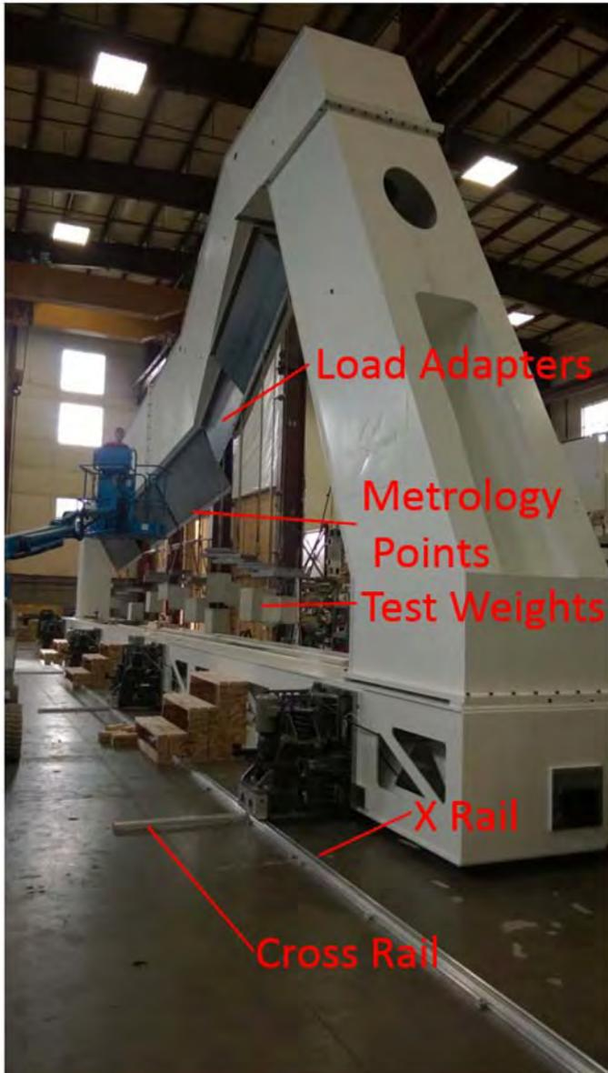
Figure 10. Physical test setup
