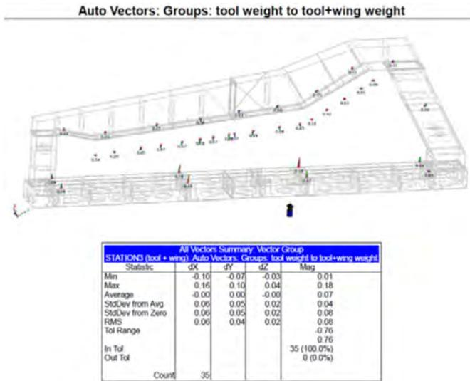
Figure 12. Spatial Analyzer results for the live load of loading the wing into the fixture (rear spar (top beam) weights only)
