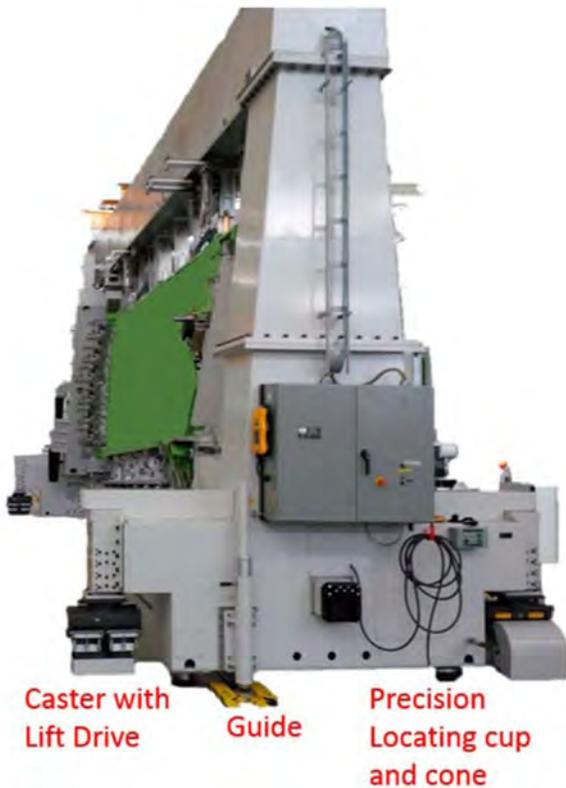
Figure 1. Alternative caster-supported system considered
