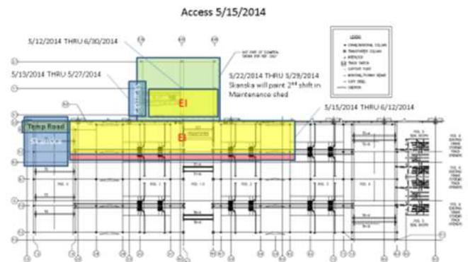
Figure 5 Example of identified control zones. Zones not colored indicated areas under the jurisdiction of concrete contractors.
