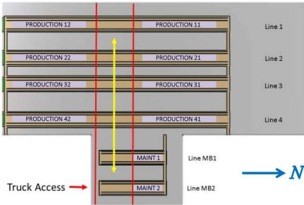
Figure 18 Machine cell layout. The yellow arrow indicates the machine transporter path.
