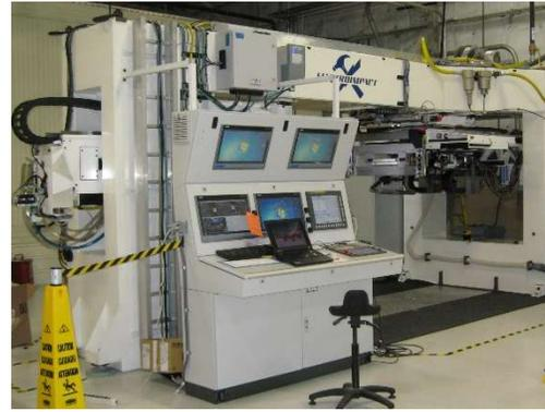
Figure 7 PAL test bench includes the operator control, process tools, shuttle table, clamp tables and vacuum system of actual production machine.
