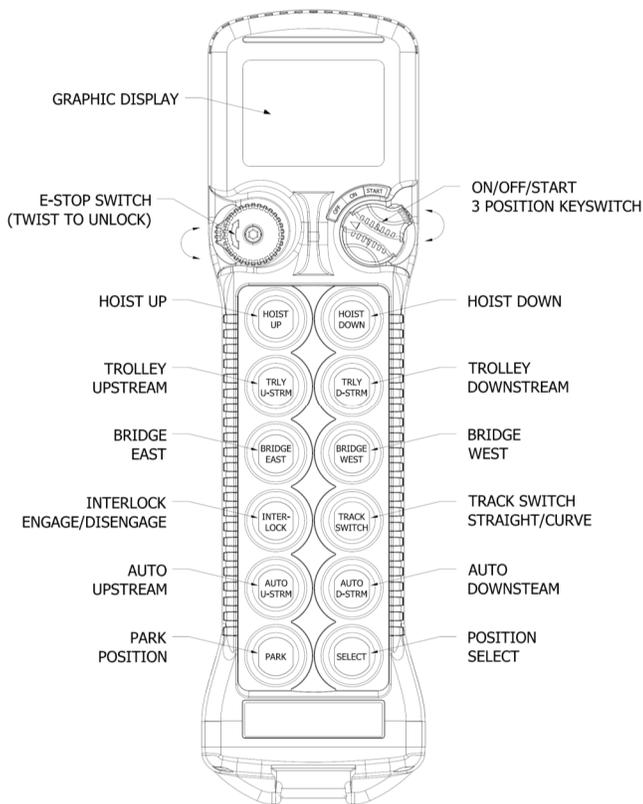
Figure 21. PAL Semi-Automated monorail has “Auto Upstream” and “Auto Downstream” buttons that allow wing panels to be moved quickly and precisely between two positions of the line.
