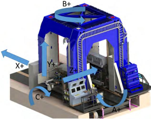
Figure 1. Vertical fastening machine overall arrangement.
