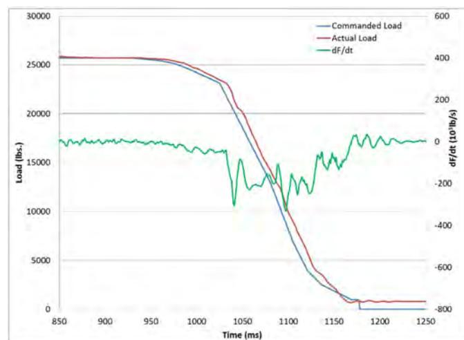
Figure 11. Reduced vibration in measured load during smoother transition from dwell to ramp down.
