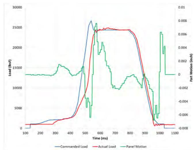
Figure 9. Plot of panel motion during upset.
