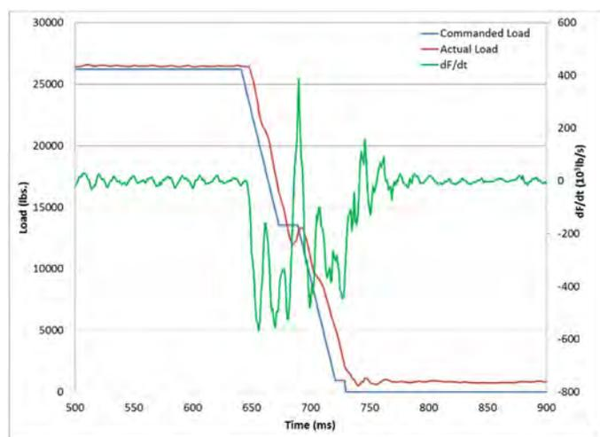
Figure 10. Vibration in measured load during sharp transition from dwell to ramp down.
