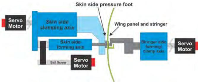
Figure 2. Mechanical upset arrangement.
