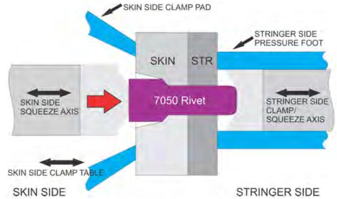
Figure 3. Rivet insertion and seating in the countersink.
