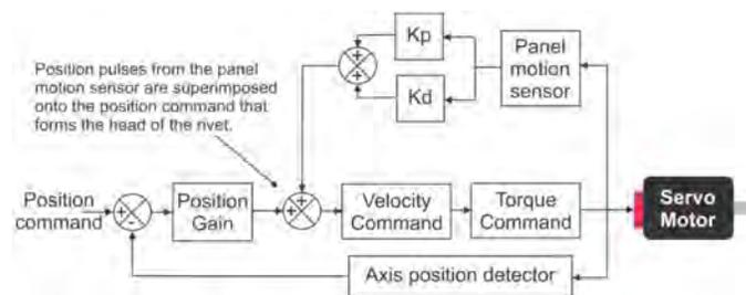
Figure 8. Skin side forming axis process control loop.
