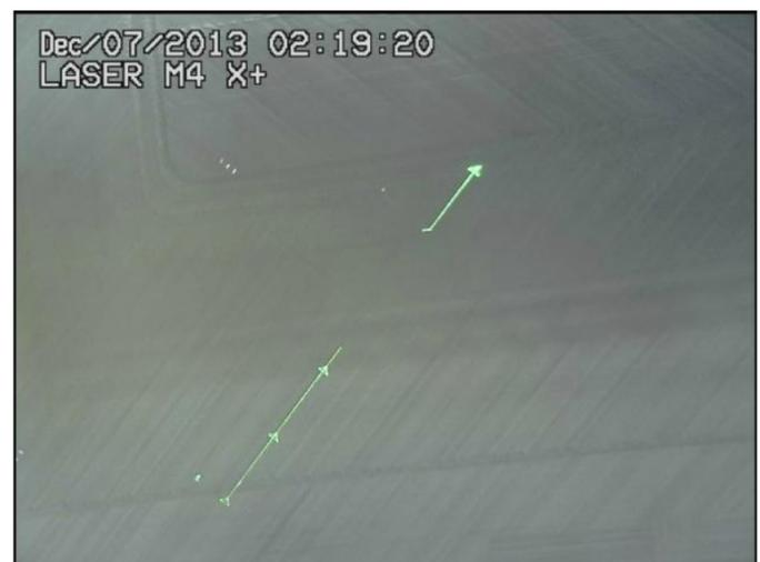
Figure 4. Laser projection of course containing logged error or user specified course
