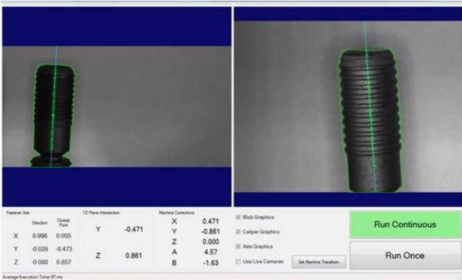
Figure 11 3D Vision of Fastener Tails
