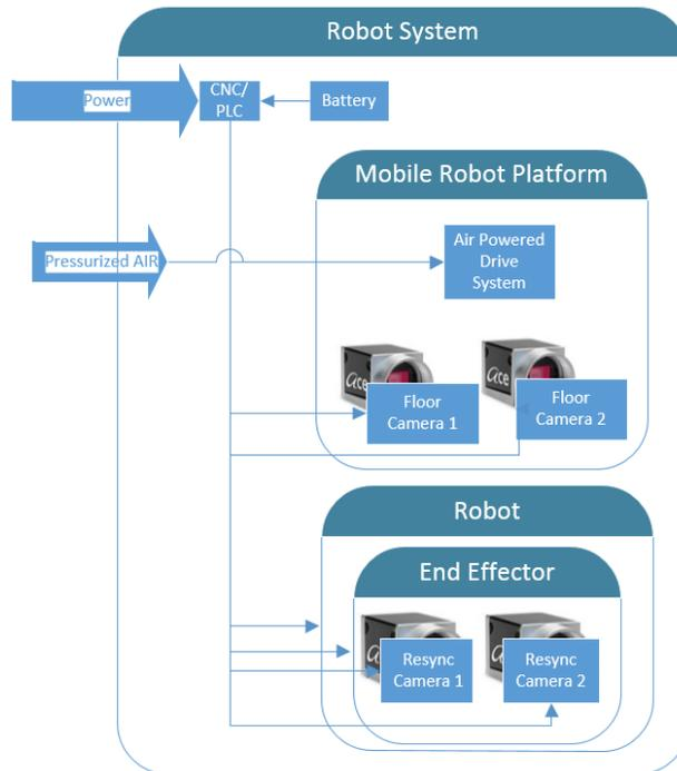
Figure 2 System Architecture
