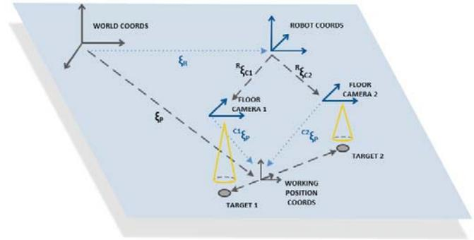
Figure 8 Transform Graph: Grey coordinate axes and grey dashed lines are static. Blue axes and blue dotted lines are dynamic.
