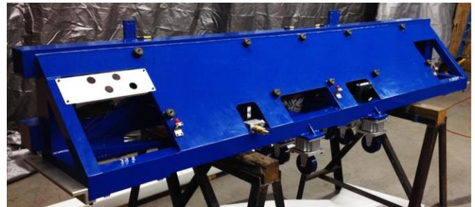
Figure 5: Machine frame rear face with aluminum "skin" prior to major machine assembly.
