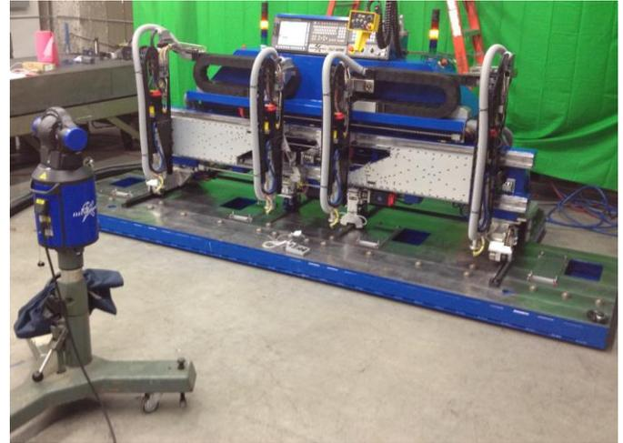
Figure 20: Laser tracking alignment plate bushings with machine mass positioned on plate.
