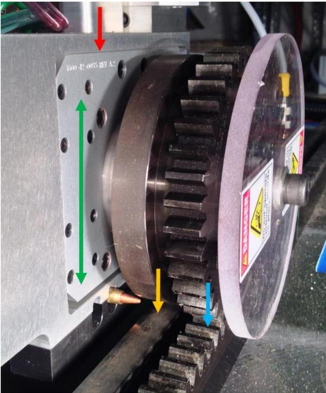
Figure 8: Waterline deviation compensation system.
