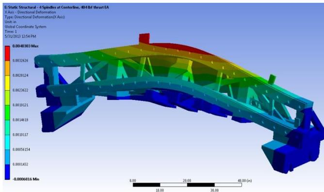
Figure 3: Frame twist on an early frame FEA model.
