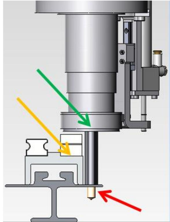
Figure 9: Chip shroud (green arrow) next to bridge track tooling (orange) while drilling the seat track (red).
