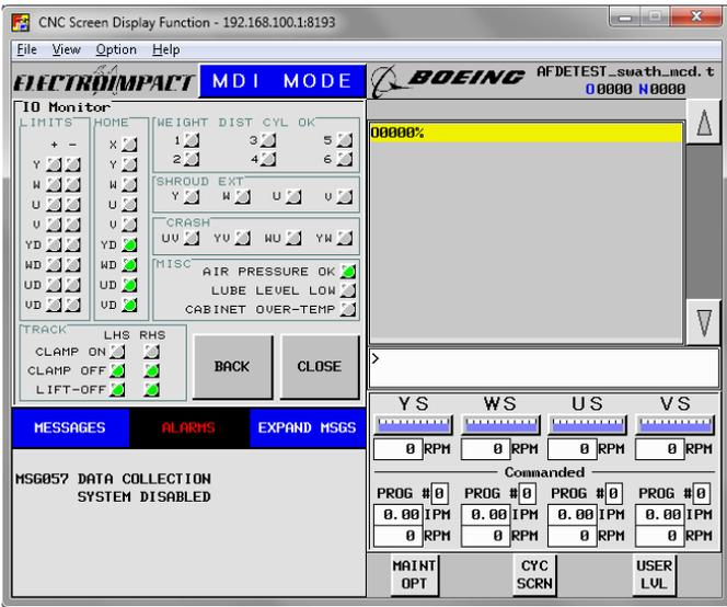
Figure 18. I/O Monitor screen.
