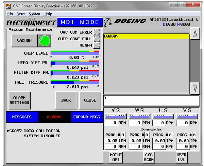
Figure 16. Vacuum maintenance screen.
