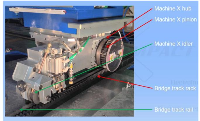
Figure 7: 767AFDE X axis drive system.
