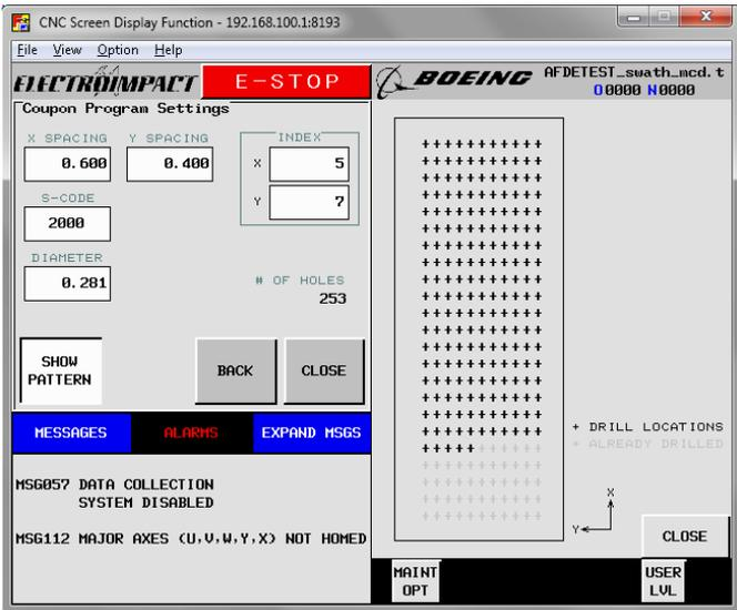
Figure 19. Coupon drilling setup screen.
