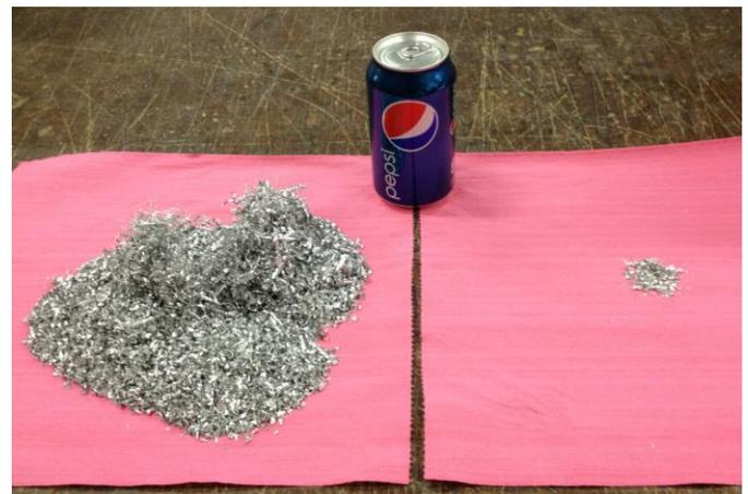
Figure 10: Chips captured in vacuum (left) versus chips left on floor (right).
