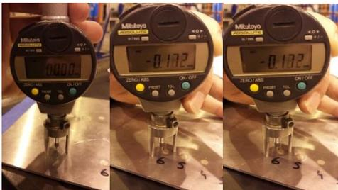
Figure 6. Measurements showing dimpling in stacks thinner than 4mm.
