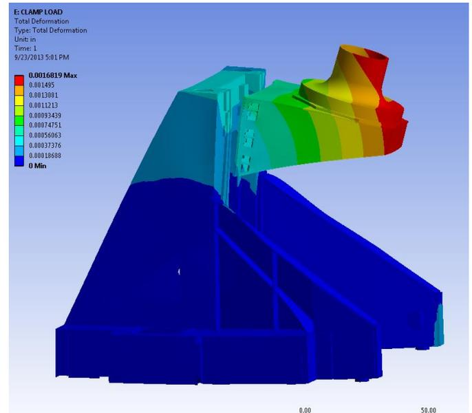
Figure 4: Plate structure gives good control of deflections
