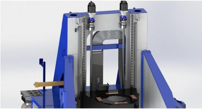
Figure 9: Dual Heidenhain absolute glass scales, mounted outboard of the Y rails
