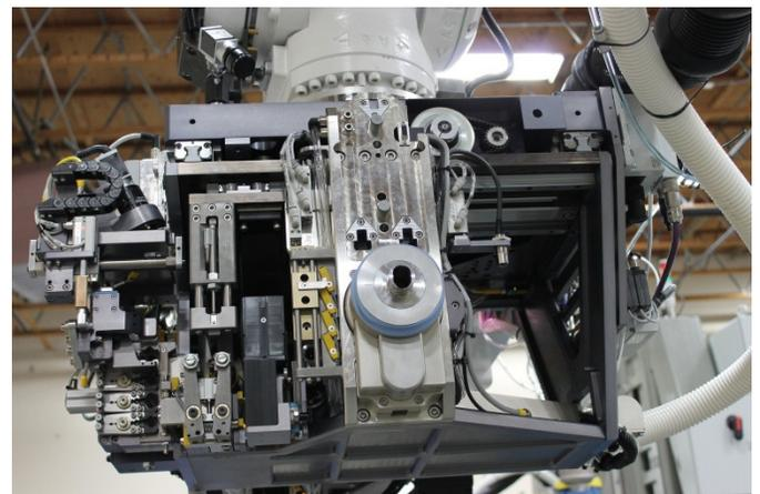
Figure 6 End Effector from Described Mobile Robot
