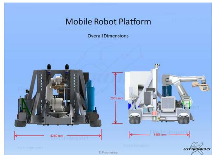
*Figure 1 - Overall Dimensions Mobile Robot*
