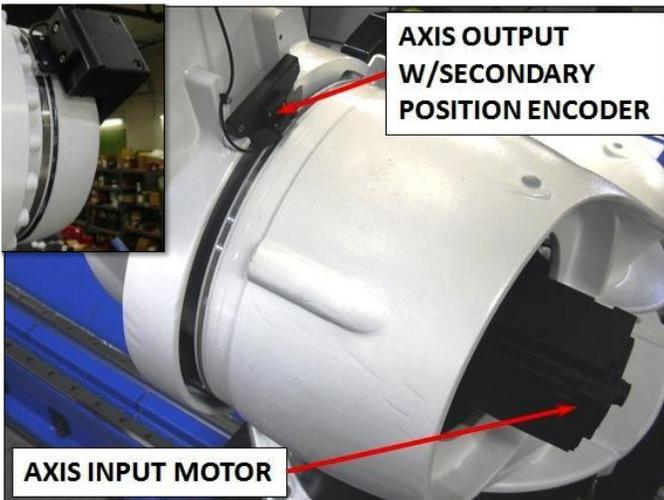
Figure 5 - Secondary Feedback
