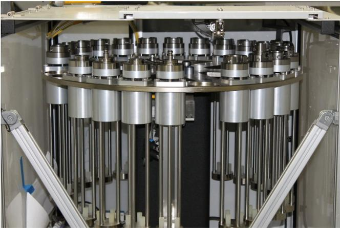
*Figure 10 Automatic Tool Changer*
