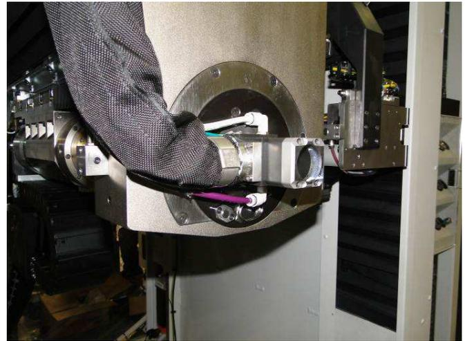
*Figure 13 Pressure Foot Nosepiece*
