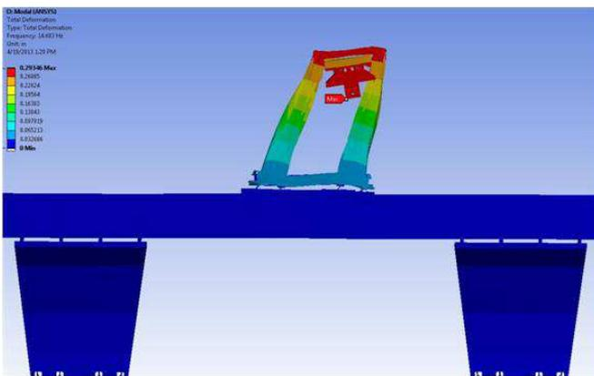
Figure 8 Second Mode of New Beam and Columns
