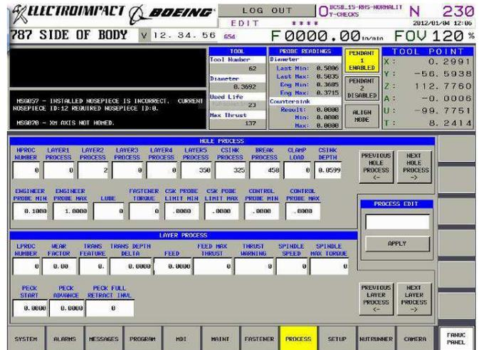
Figure 11 Drill Process Screen
