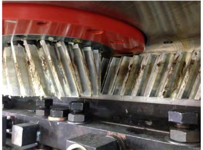
**Figure 4.** Rack and pinion drives require grease that must be isolated from the clean room environment.
