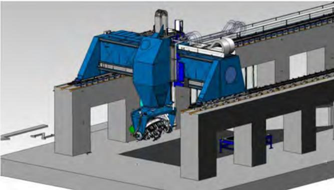
**Figure 2.** A “high rail” gantry system eliminates the need for heavy structural legs.
