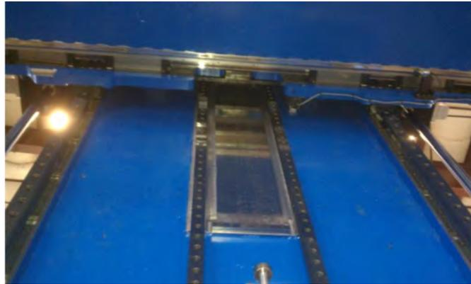
**Figure 5.** Attraction forces are reacted with linear rail locally around magnet plates.
