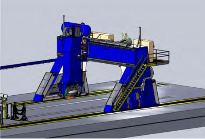
**Figure 1.** A traditional “high leg” gantry AFP positioner increases moving mass to allow for a large working envelope.
