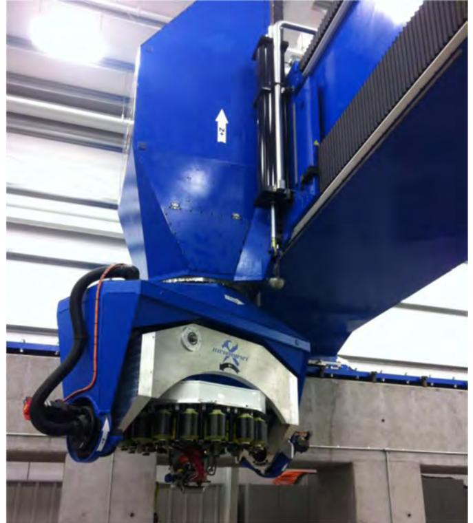
**Figure 10.** two large pneumatic cylinders work in conjunction with a large accumulator to counterbalance 100% of the mass of the vertical z-axis.
