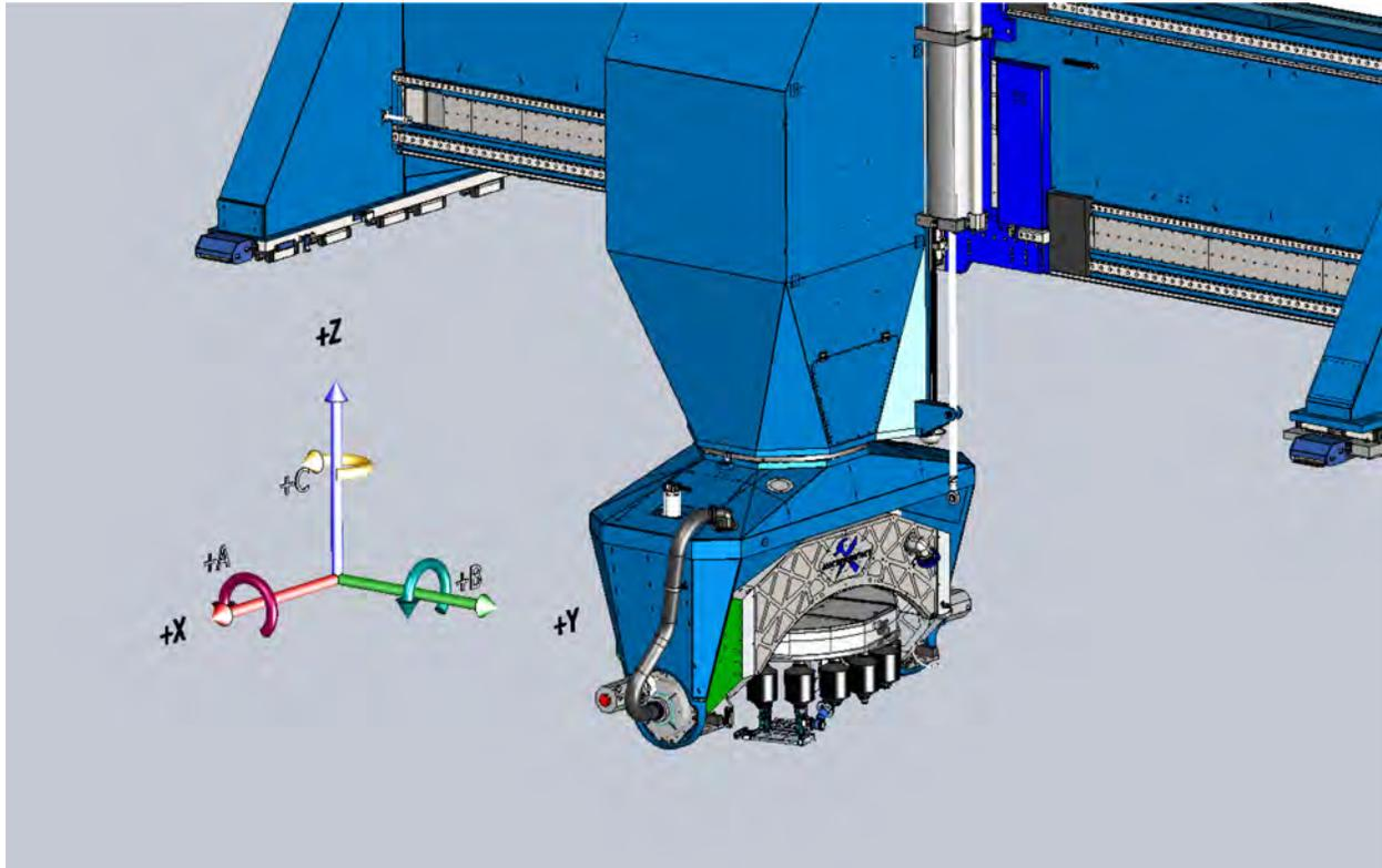
*Figure 11. Machine axis coordinates.*
