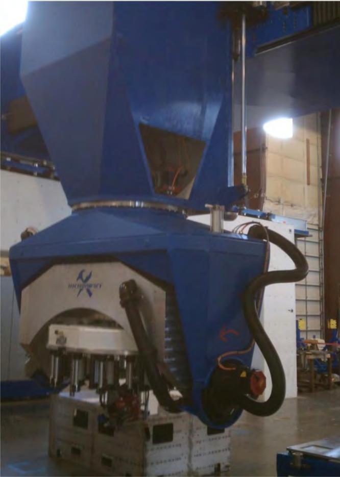
**Figure 9.** By utilizing a 210 degree range of motion, a C-prime axis effectively allows for 180 degrees of B-axis rotation.
