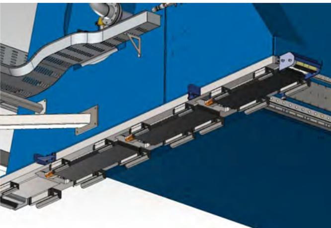
**Figure 6.** Multiple linear motors are used on the same axis to improve machine top speed and acceleration.
