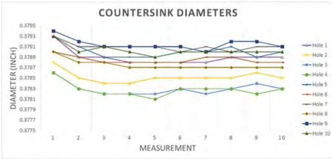
**Figure 9. Series of 10 consecutive Countersink Diameter Measurements**
