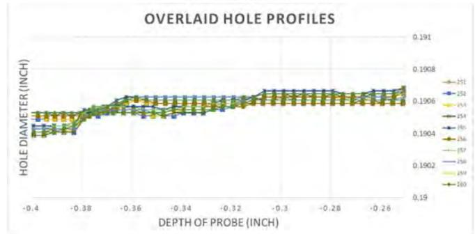
Figure 8. Series of 10 consecutive hole probe measurements zoomed in for clarity
