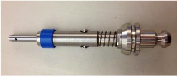
**Figure 2. Typical quick-change assembly with bore gauge and countersink measurement.**
