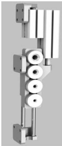
**Figure 3. Proving ring selector allows calibration of hole probe concurrently with drilling.**
