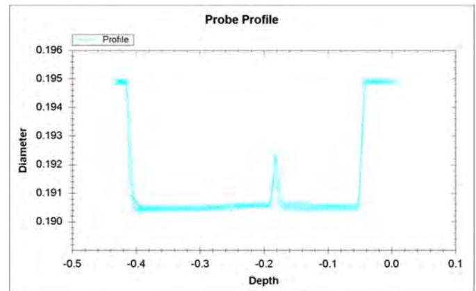
**Figure 4. Example hole profile of 0.4" stack-up of 2 plates with a 0.020" gap.**
